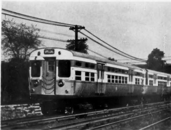
**IMPROVED DESIGN** of control and motors gave lightweight rapid-transit cars more horsepower per pound at little weight increase.
