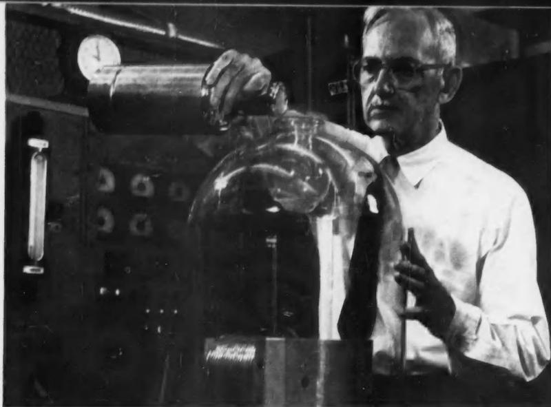
**VOLTAGE-TUNED MAGNETRON**, tuned by varying the d-c supply voltage, permits much faster tuning and therefore the use of magnetrons in many new automatic testing devices.
