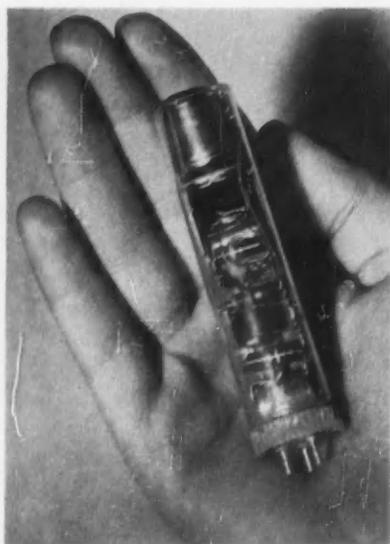
**TRANSISTOR** micropower audio-frequency amplifier can operate for three years.
