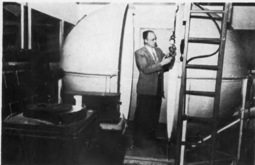
STANDARD LAMP FROM BUREAU OF STANDARDS CALIBRATES LUMINAIRE TEST LAMP.
