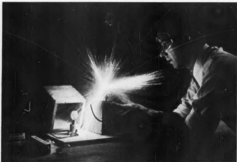
**ZIRCONIUM METAL POWDER**—heat-sensitive ingredient in a primer—ignites readily, resists oxidation in an oxygen atmosphere at normal temperatures, and can be handled safely.
