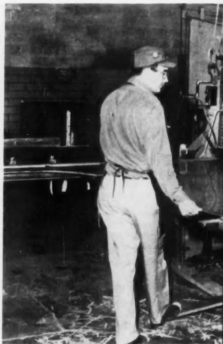
**5** A separated four- by eight-foot Textolite laminate is now trimmed of all its rough edges on a giant shear cutter. Next, its smooth
