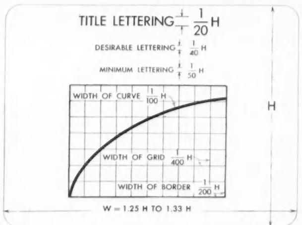
**SCREEN READABILITY** of printed matter requires specific letter sizes and line widths in relation to their projected reduction.
