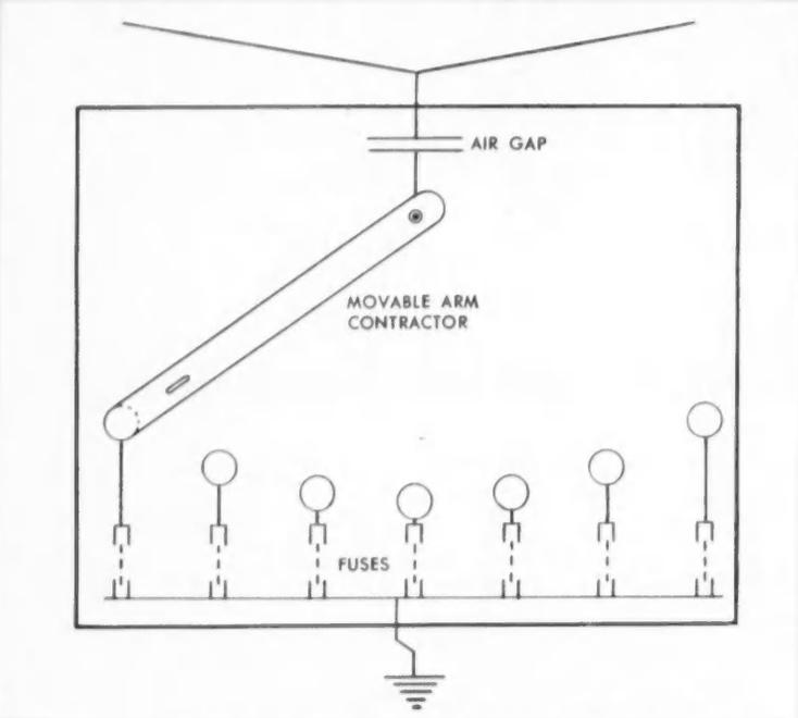
FIG. 5. FUSE LIGHTNING ARRESTER
