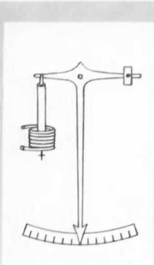
FIG. 2. AMMETER OR VOLTMETER
