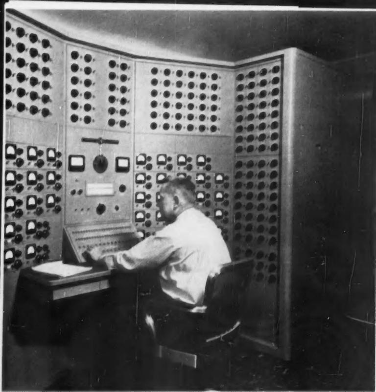
**PENALTY-FACTOR COMPUTER** applied to AG&E system saves over \$100,000 a year compared to operating the system with transmission losses neglected.
