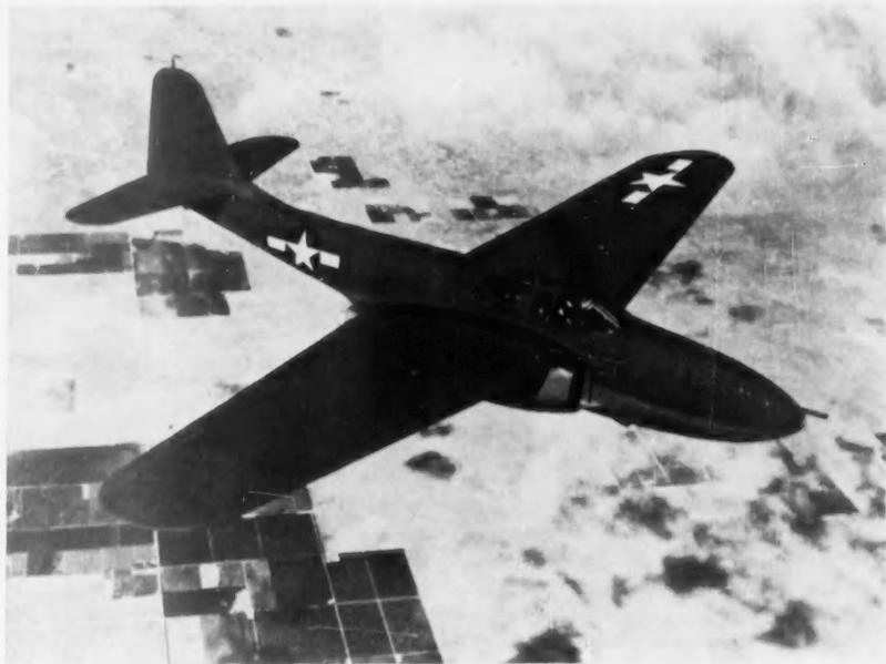
**BELL P59 AIRACOMET**, propelled by two of the first American-built turbojet engines, zipped through the air on October 2, 1942. Each of its engines delivered 1250 pounds of thrust.
