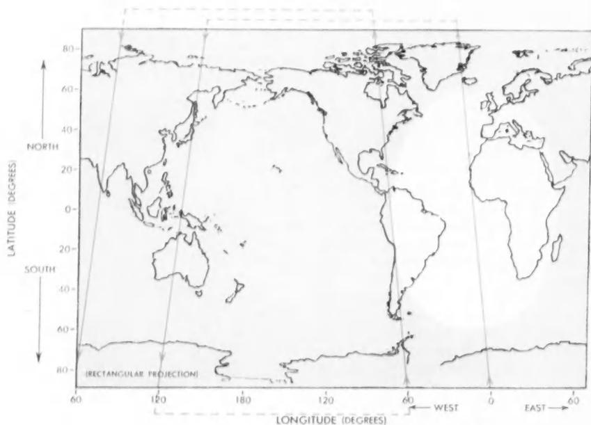
Two successive tracks of a satellite 300 miles out in space, moving west to east on an orbit inclined 40 degrees to the equator, can be graphically shown (illustration, top). Actually, the satellite travels in space about 96 minutes. But when viewed from the earth—also moving west to east—its *apparent* period is about 104 minutes.
