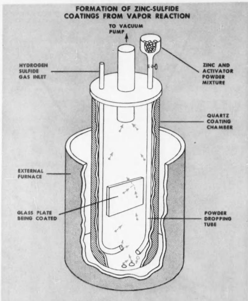
VAPOR-DEPOSITION METHOD produces phosphor layers having desired characteristics.
