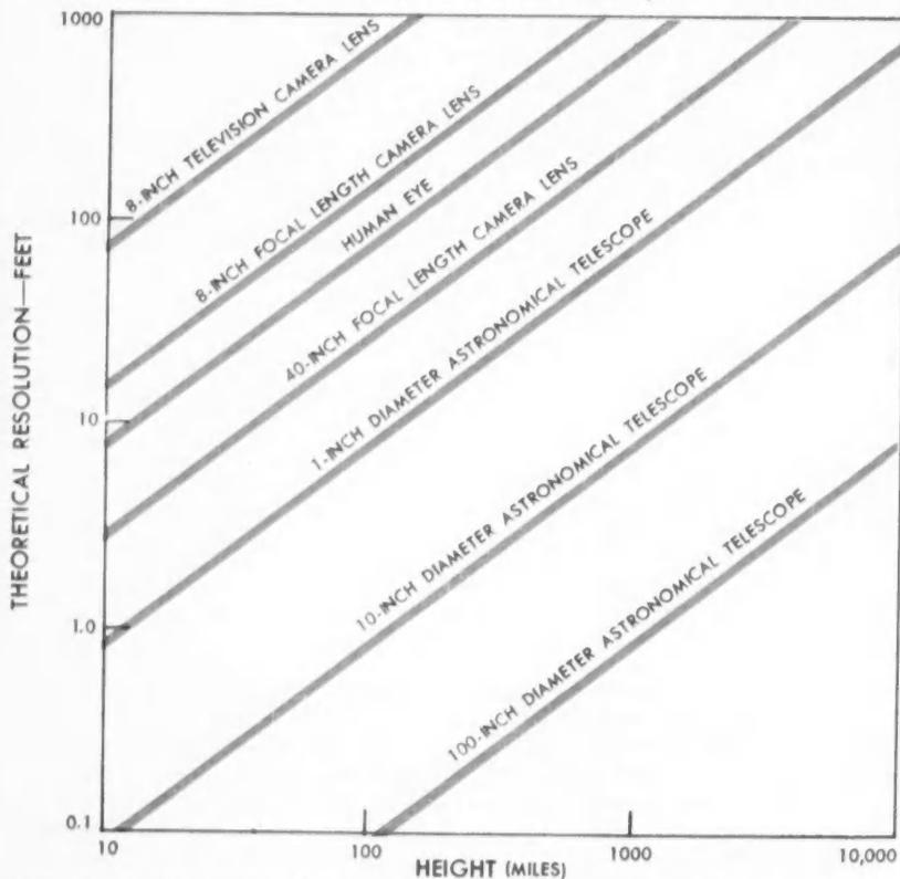
**LENS SYSTEMS** limit ability of cameras to resolve detail at great distances. The eight-inch focal-length camera lens is representative of the type now used to make aerial surveys.
