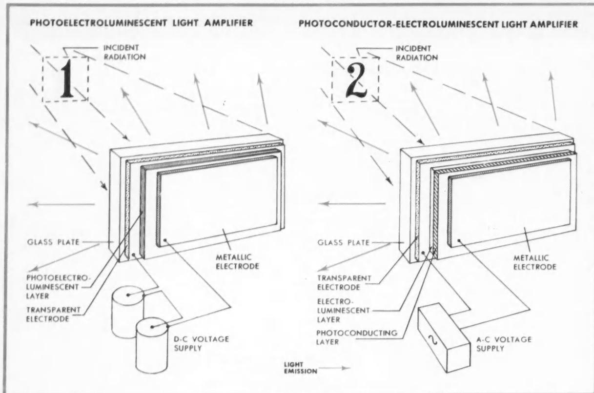
**INCIDENT RADIATION** initiates and controls light emission. Amplifier (right) utilizes two well-known solid-state elements.
