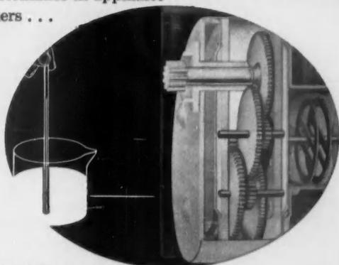
**BECAUSE** capillary action feeds oil to moving parts. The oil, drawn up between the plates, furnishes a continuous source of lubrication for all bearings.
