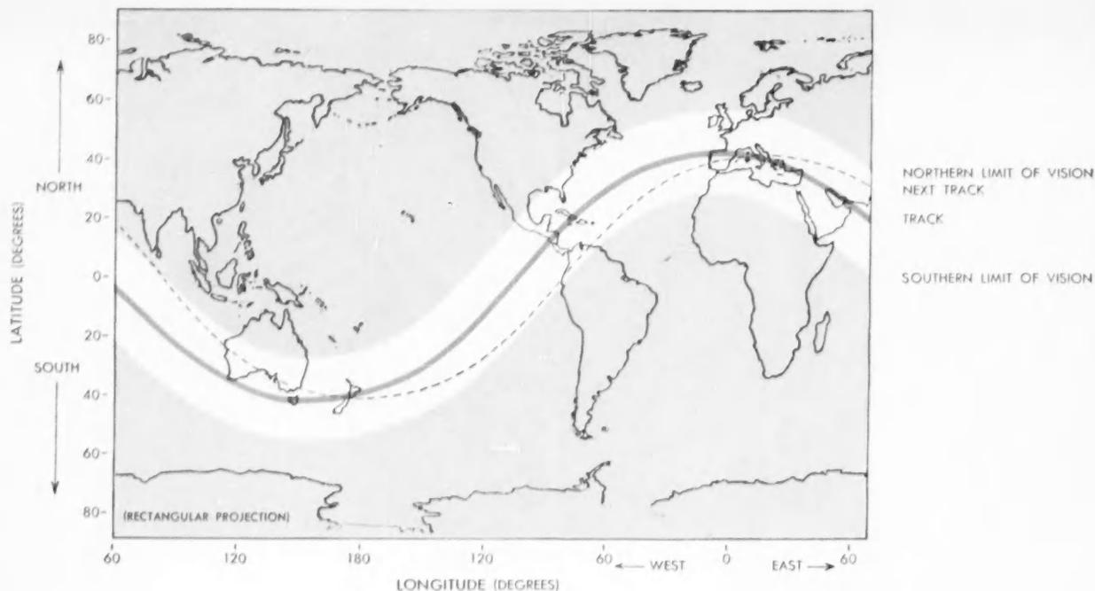
Earth mass as seen from a satellite 300 miles high and traveling eastward in its orbit changes with each successive track (above). Twice in 24 h urs, every point on the earth's surface would be visible from a 1200-mile-high satellite orbiting around the poles (right).
