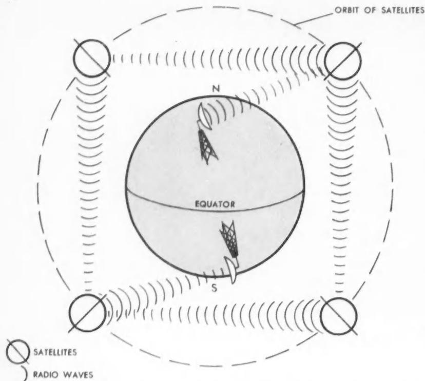
**FOUR SATELLITES** equally spaced on a 1000-mile-high equatorial orbit provide an excellent communications link. Signals transmitted from earth can be relayed around the world.
