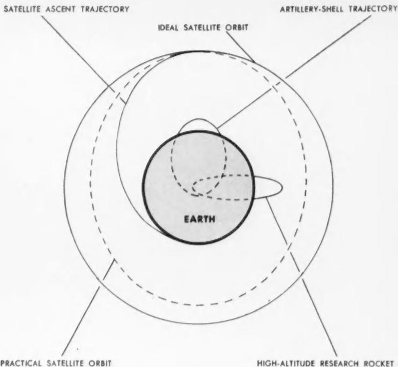
**TRAJECTORIES** of bodies fired from surface of earth follow elliptical paths with one focus at earth's center. Planets also orbit elliptically but with the sun at one focus.
