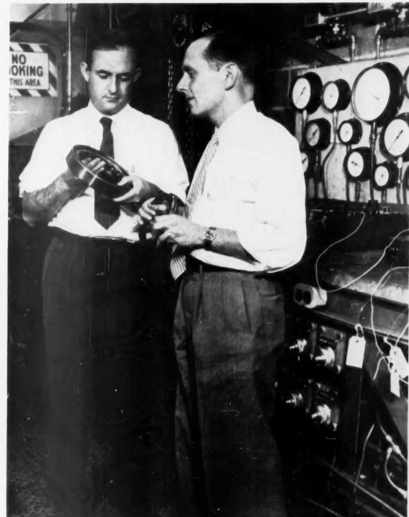
**BALL BEARING** used to support compressors in jet engines is being examined by authors Jackson (left) and Booser after test-running the bearing at a temperature of 700 F.
