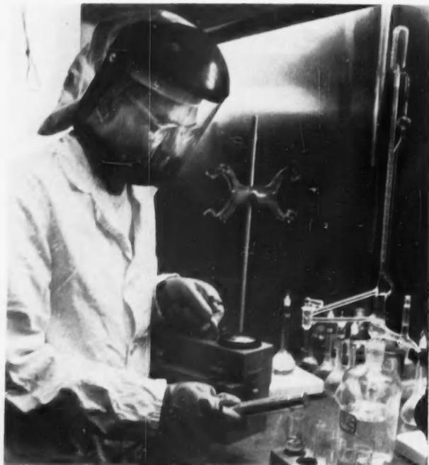
**RADIO CHEMIST** monitors radioactive solutions beneath exhaust hood during an analysis for traces of nuclear fission products. Note the plastics radiation-detecting rings on his index fingers.
