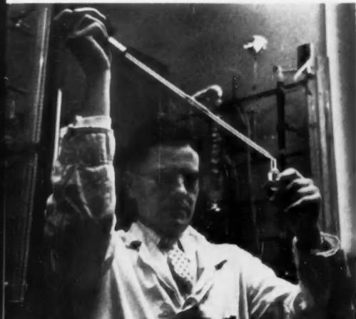
**4** Once inside his own laboratory, he prepares a solution for irradiation by specific amounts of gamma rays. In this way, Dr. Jones can determine their physical and chemical effect.
