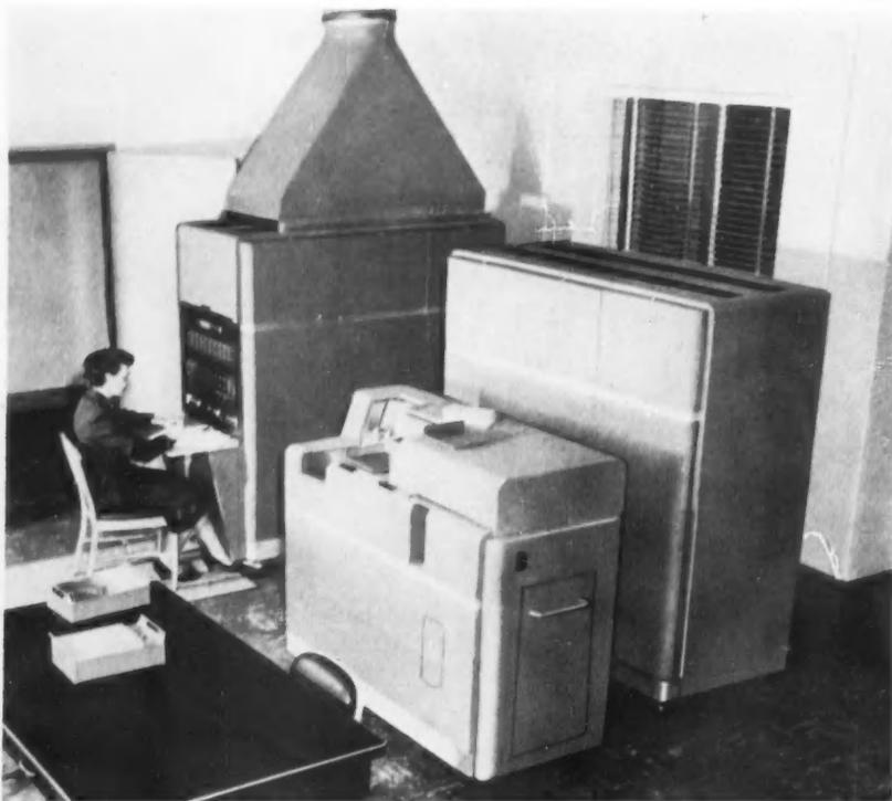
**LARGE-SCALE DIGITAL COMPUTERS**, such as the IBM 650, are being manufactured on production lines by the hundreds and find use in scientific and engineering computation, as well as financial, statistical, operations research, and similar data-processing activities.
