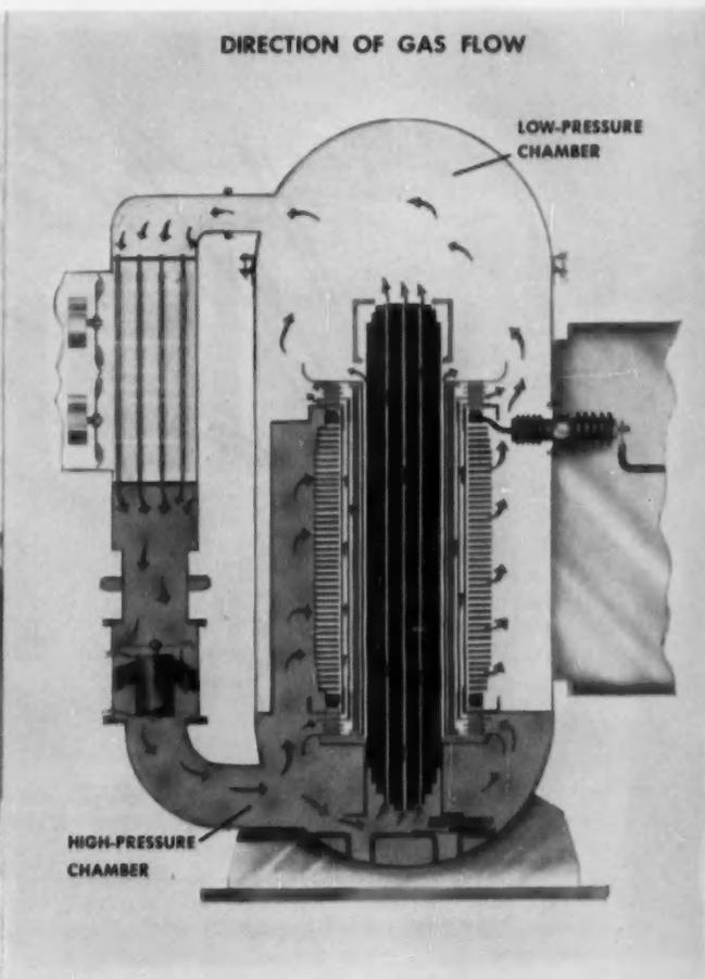
PROTOTYPE OF GAS-INSULATED SINGLE-PHASE 1000-KVA TRANSFORMER IS EXAMINED BY AUTHOR (RIGHT); GAS FLOWS IN ARROWED PATHS.
