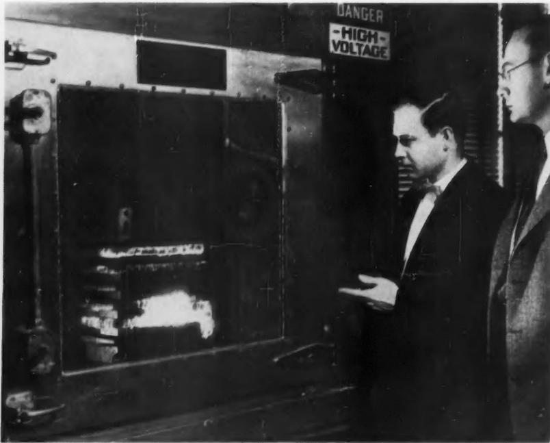
**TORTURE CHAMBER** duplicates and accelerates severe service conditions in the laboratory. Authors Norman and Thompson observe surface sparking on molded instrument transformer.
