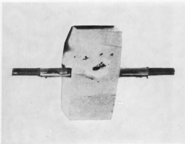
HIGH VOLTAGE APPLIED TO THE ELECTRODES CAST IN BUTYL RUBBER (CENTER) CHARNS A CONDUCTING PATH BETWEEN THEM. BUT WITH NON-
