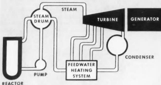
**STEAM FLOWS FROM REACTOR** to drum. Saturated steam passes to turbine; water goes to feedwater heaters and returns to steam drum. Forced circulation pump provides automatic control of response to load changes.
