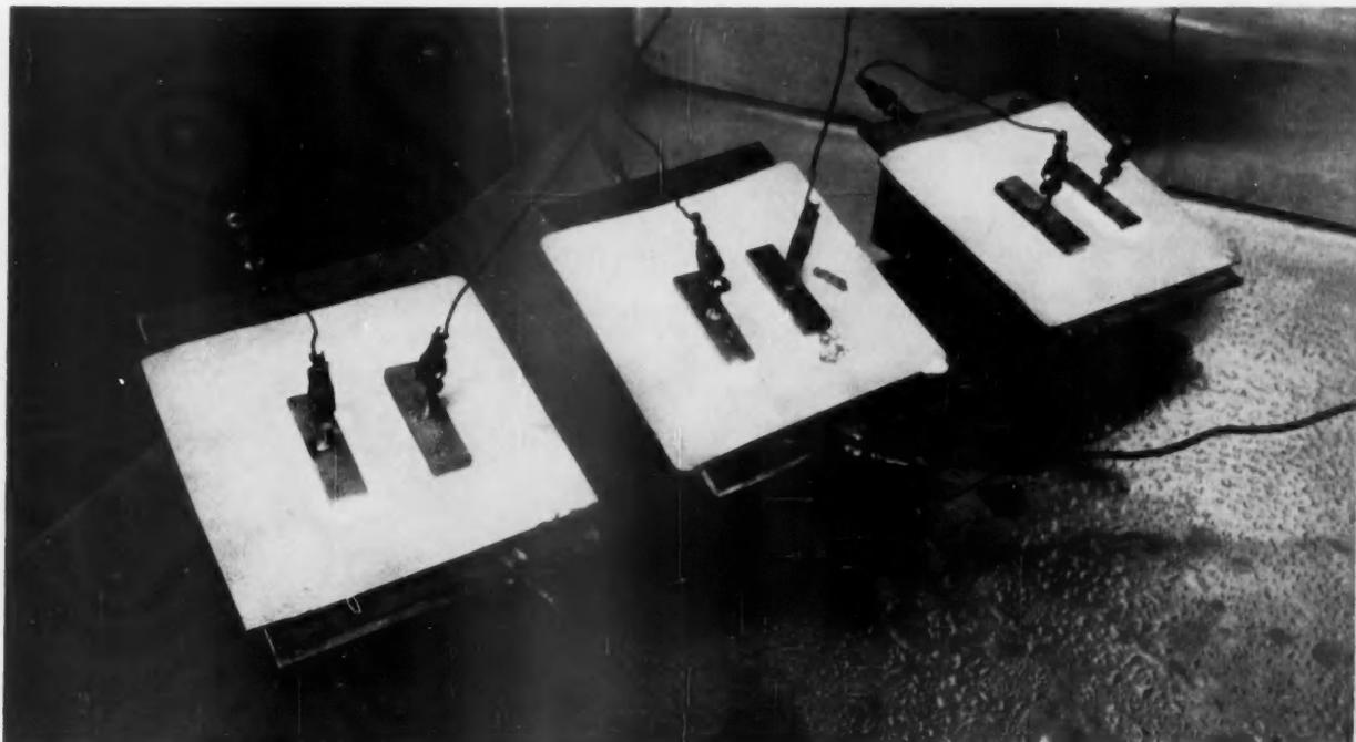
INSIDE FOG CHAMBER, NONTRACKING INSULATION COVERED WITH SYNTHETIC DUST COUNTERS THE FORMATION OF FREE CARBON.
