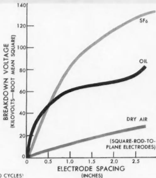
**GASEOUS FLUOROCOMPOUNDS** have progressed to the point where they now have a fairly high dielectric strength at moderate pressure.
