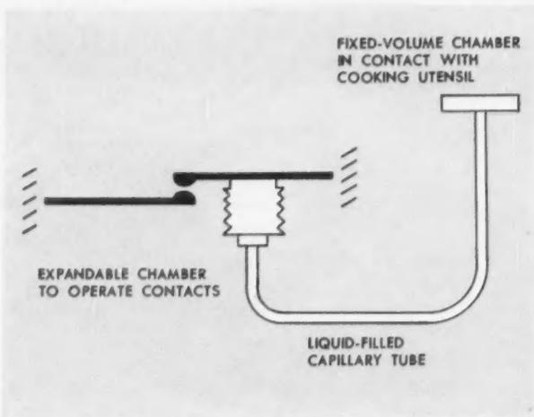
TEMPERATURE-SENSITIVE DEVICE (ARROW) OPERATES ON THE PRINCIPLE THAT LIQUID VOLUME VARIES WITH TEMPERATURE CHANGE.
