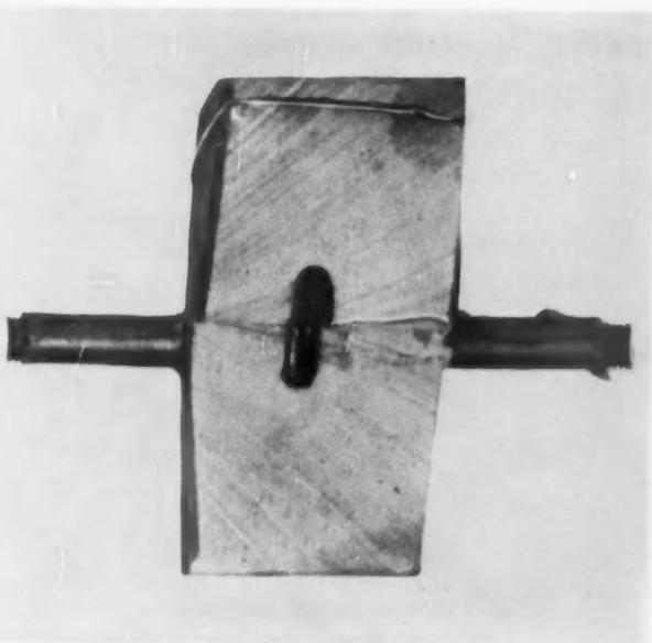
TRACKING INSULATION (RIGHT), NO CARBONIZED PATH FORMS.
