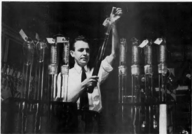
**ASTM OXIDATION TEST** for turbine oils is prepared by the author. The test has been modified in the laboratory to obtain preliminary information concerning the test samples.
