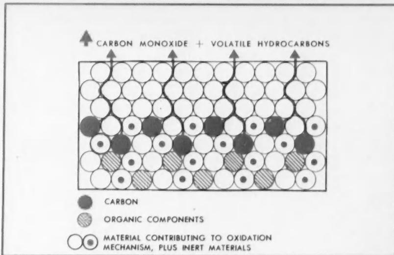
CARBON MONOXIDE AND GASEOUS HYDROCARBONS ARE FORMED INSTEAD OF FREE CARBON.
