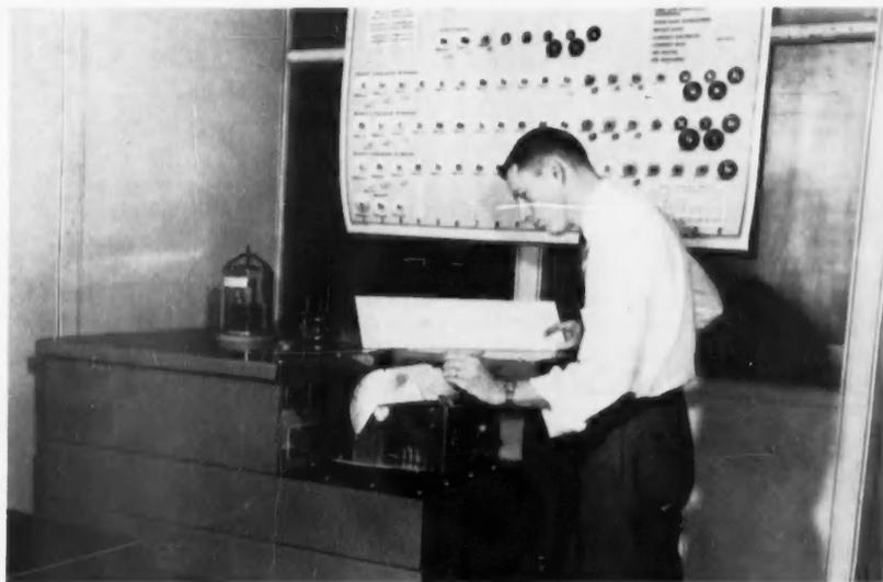
INFRARED SPECTROPHOTOMETER HELPS ESTABLISH COMPOSITION OF NONMETALLIC MATERIALS.
