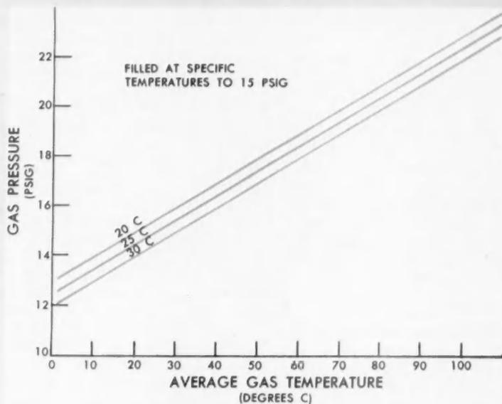
**PRESSURE OF A GAS** varies with its temperature, but the dielectric strength of sulfur-hexafluoride gas is independent of temperature if its density remains constant.
