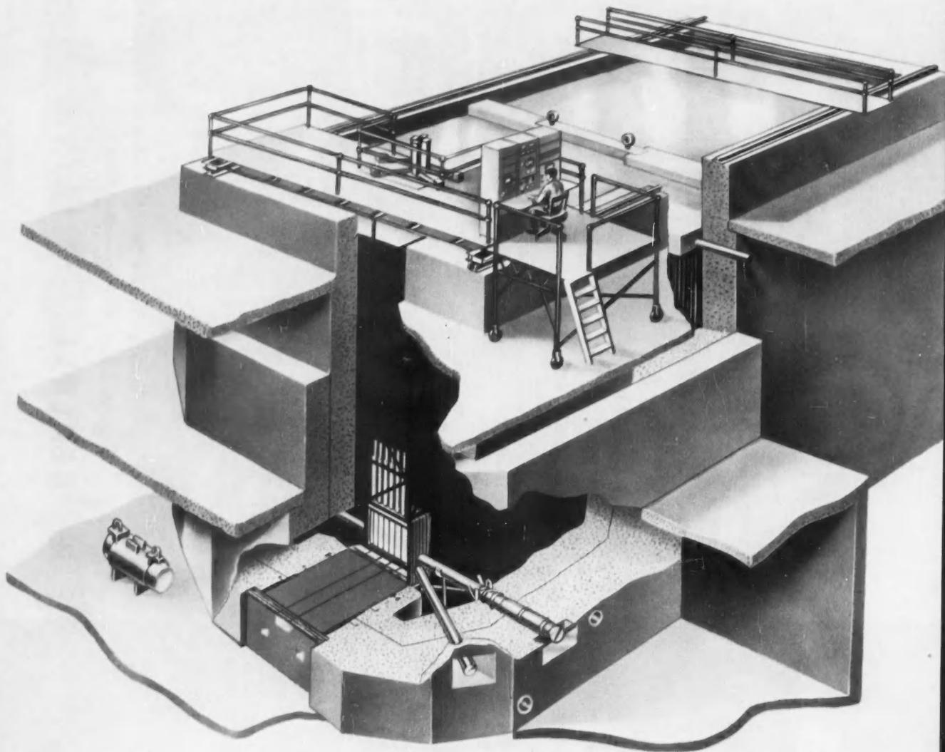
**SWIMMING POOL REACTOR**, one of three G-E research reactors available under the 7-point program, is designed to produce large quan-
