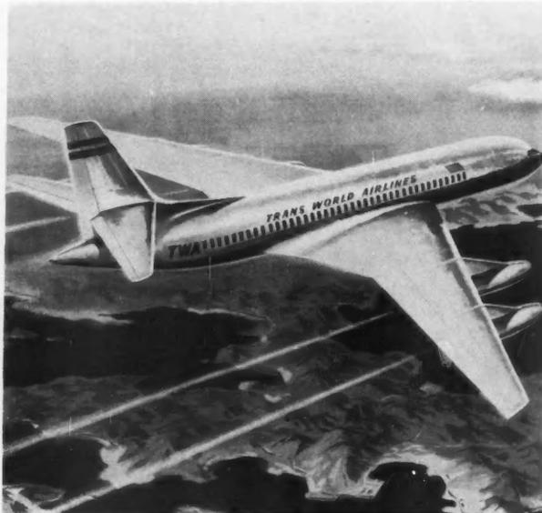
LOCKHEED'S F104A *Starfighter* is powered by J79 turbojet engine and a commercial version of the J79 will propel the Convair 880.
