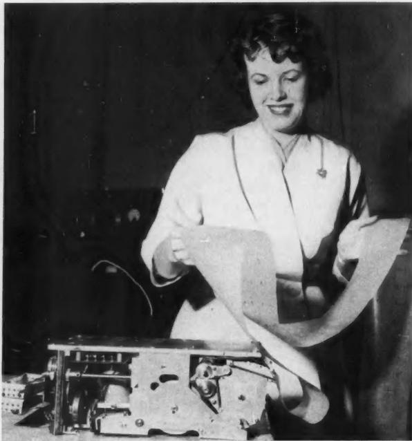
**HIGH-SPEED** mechanism prints more than 2500 lines per minute.
