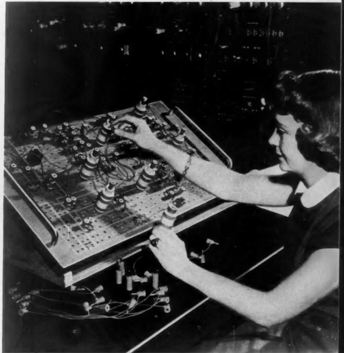
**ANALOG COMPUTER** investigates locomotive systems' stability and transient response and solves heat-transfer and design problems.
