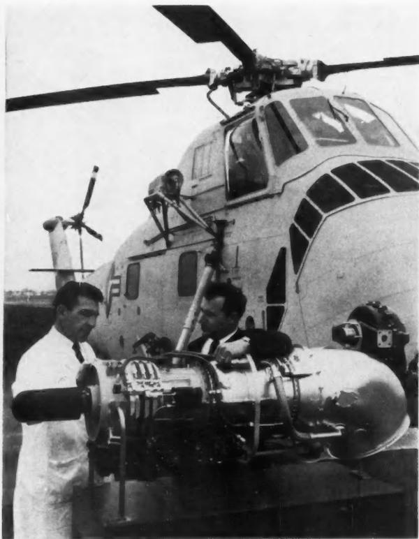
**TURBOSHAFT ENGINE**, the T58, will soon be flying in helicopters.
