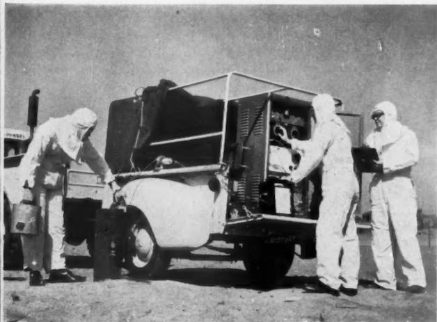
**PROBE** and related equipment quickly detect radioisotopes in soil.
