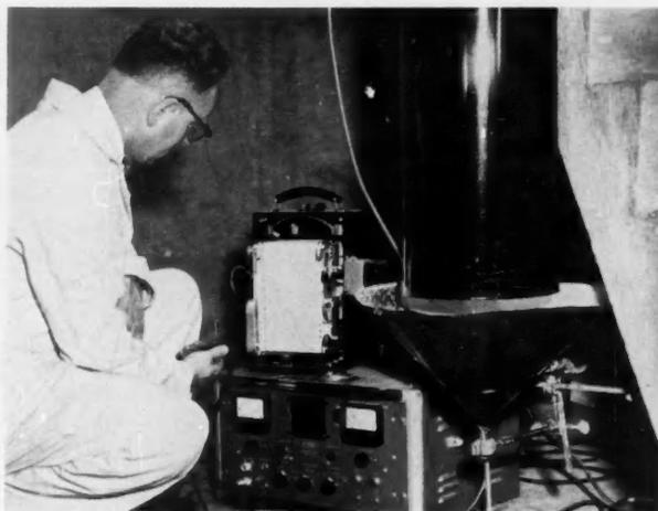
**TERMINAL VELOCITY** of particles is measured by counting meter.
