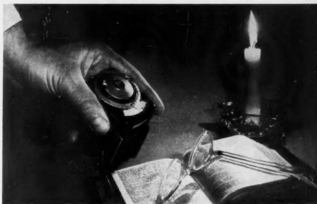
**LIGHT-MULTIPLIER ATTACHMENT** boosts the sensitivity 64 times on a new mass-produced photographic exposure meter.
