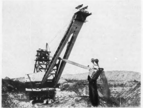
**ELECTRIC SHOVEL**, standing 16 stories high and weighing 2700 tons, can take a 90-ton bite of earth and drop it up to 300 feet away.
