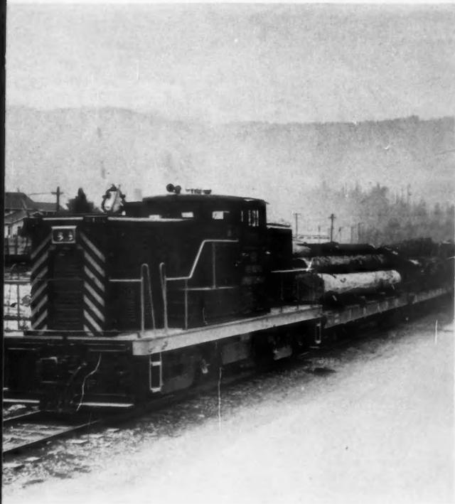
**INDUSTRIAL LOCOMOTIVE**, newly added to the standard diesel-electric line, produces a total of 840 hp for traction purposes.
