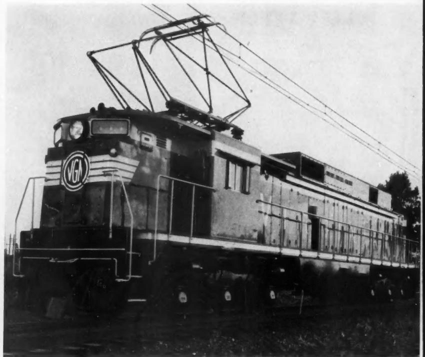
**RECTIFIER-TYPE LOCOMOTIVES** entered a new field in the fall of 1956 when the first of 12 units went into heavy freight service hauling coal trains on the Virginian Railway.
