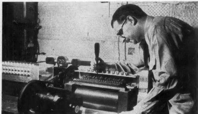
**METAL CYLINDER**, possessing an over-all capacity as high as 3-million bits, supplies computer with information needed to solve problems.
