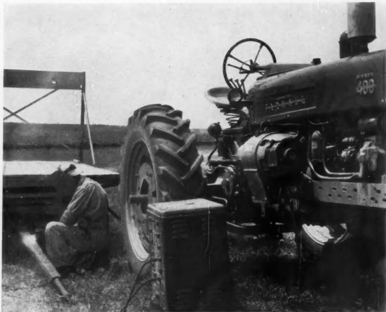
**Welding** Damaged equipment that normally would have to be taken to town for repairs can, with the aid of the mobile generator, be fixed in the field.
