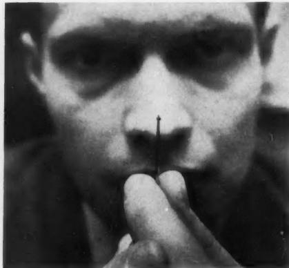
**MAGNETIC CORE** (impaled on a needle) is capable of storing one bit of information.
