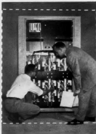
**NEW DESIGN**—Smaller size, greater dependability, and lower cost are the features of this new cubicle design. Dotted outline shows the former size. New design is 44% smaller, yet delivers 20% more power output.
