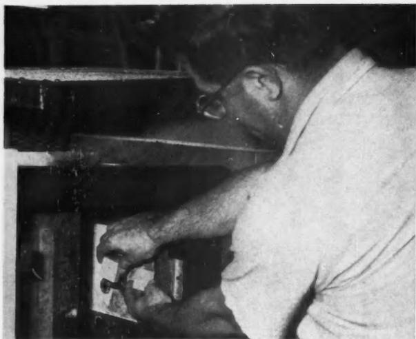
**5** Automatic molding cycle completed, operator raises safety gate and reaches in to remove plastics part from open mold.
