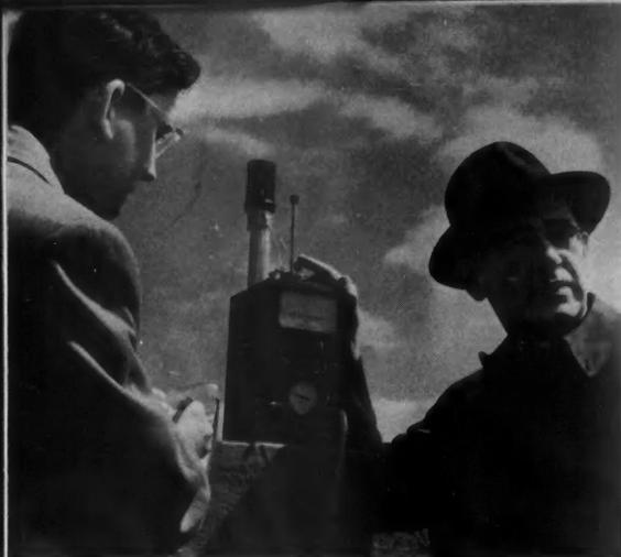
Comprising haze that overhangs industrial complex (left) are airborne particles that Van Luik and Rich (above) measure with a portable condensation nuclei meter. Engineers (right) determine erosion rate of motor-starter contacts in test chamber.
