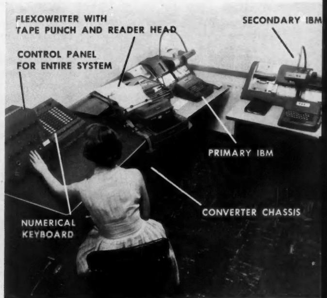
**SPARE-PARTS AUTOMATION SYSTEM** utilizes punched cards, tape, or keyboard inputs and produces typed documents.
