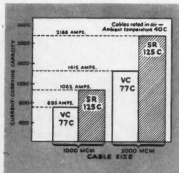
Fig. 2: COMPARISON OF CURRENT-CARRYING RATINGS—Varnished cambric vs silicone rubber cable. Based on 9 cables in duct bank, 100% load factor, 25 C earth, open-circuit sheath.
