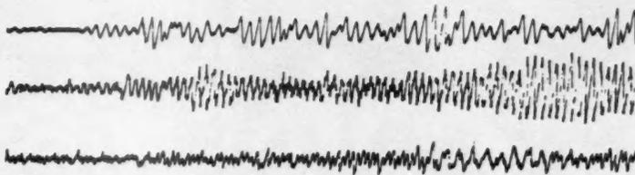
**VIBRATION PATTERNS** of blades show low stresses of normal, unstalled operation (left) and the high stresses that occur during a stalled condition. Vibrations were traced of first- and fifth-stage rotor blades and fifth-stage stator vane (top to bottom).
