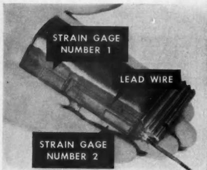
Vital to jet-engine advancement, the highly sensitive strain gage (above) tackles the task of measuring vibratory stresses of turbine and compressor blades during engine operation. Magnetic-tape recorder aids in stress evaluation. Author stands at left.
