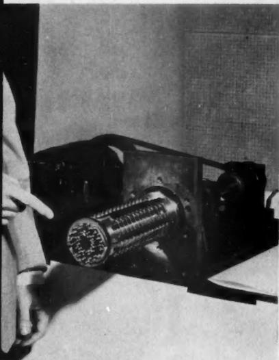
**SLIP-RING ASSEMBLY** is vital component in circuitry that records blade vibrations.
