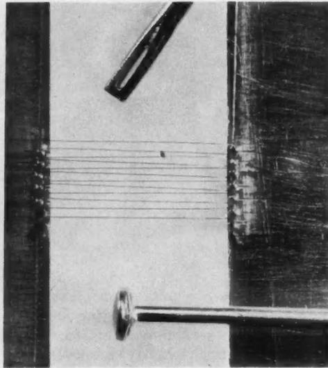
**TINY STRAIN-GAGE GRID** is formed by winding strain-sensitive wire around mounted pins—a technique requiring a great deal of manual dexterity and patience. The grid magnification (right) graphically compares the size with relation to a needle and pin.
