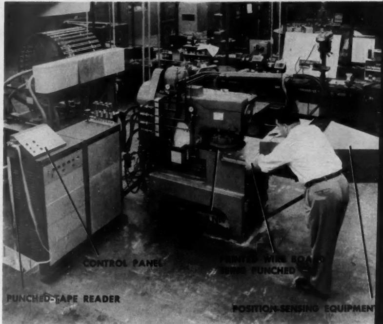
**TAPE-READER AND PUNCHING MECHANISM** quickly revises data from the original tape. New and other unchanged data from the original are punched simultaneously.
