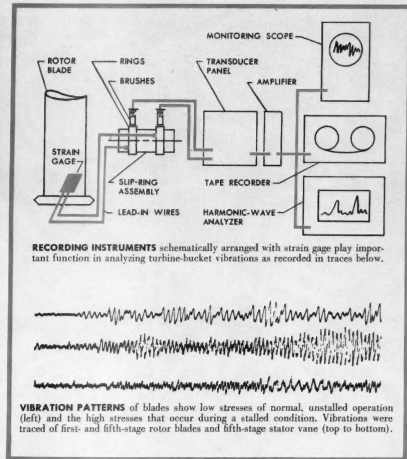
**RECORDING INSTRUMENTS** schematically arranged with strain gage play important function in analyzing turbine-bucket vibrations as recorded in traces below.
