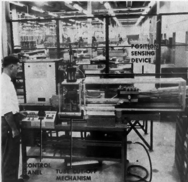
**SQUARE-TUBE CUT-OFF MACHINE** automatically cuts square hollow tubes to appropriate lengths for assembling into electronic chassis.
