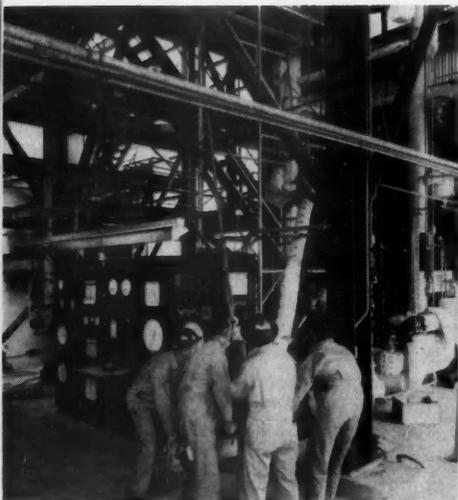
**HEAT TRANSFER AND FLUID FLOW** are tested in this special test loop designed for study of void distribution, steam slip, steam blanketing and heat transfer.
