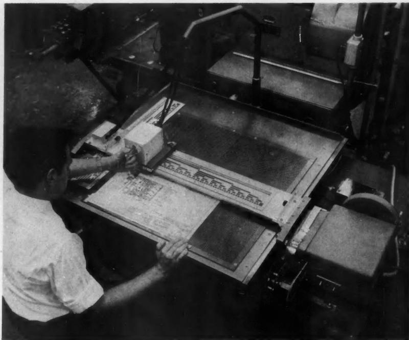
**DRAWING-TO-TAPE PROGRAMMER** automatically converts information to a common language tape. Operator merely aligns drawing on the programmer, sets selector switch for the proper hole size, and depresses the stylus beneath his thumb at the proper hole location.
