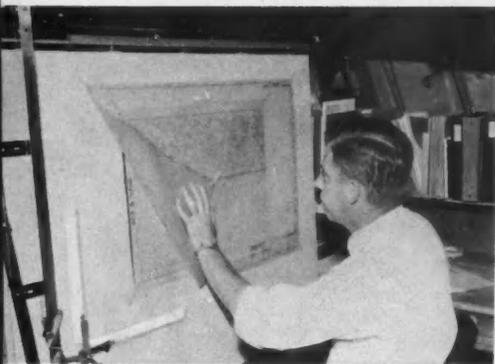
A tenth-inch incremental grid drawing (above) serves as basis for mechanized fabrication and assembly of wiring boards. Prepared from a dimensionless drawing, it's one of many new concepts in an automation program of integrated mechanization.
