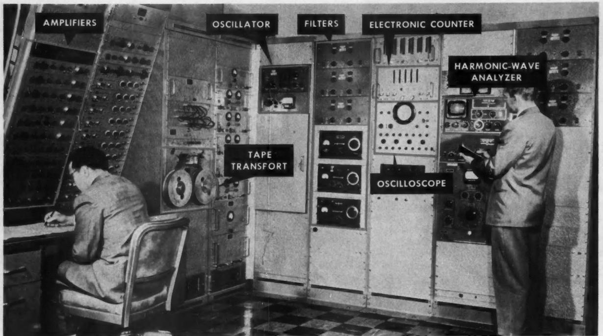
**INSTANT PLAYBACK** of data recorded on magnetic tape simplifies analysis of vibratory stresses, offering a tremendous advantage in jet-engine and missile testing. Skilled technicians utilizing a complex group of instruments interpret the data.
