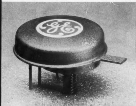
**HIGH-POWER** silicon transistor has a grounded emitter cutoff frequency of 400 kc.
