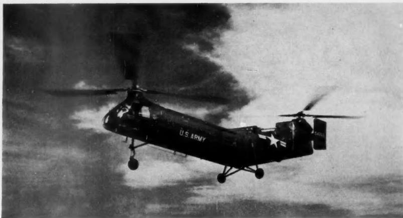
**T58 TURBOSHAFT ENGINE** powered the Vertol H21D (shown) and a modified Sikorsky S58—the first twin-engine helicopters in U.S. to be propelled by aircraft gas turbines.
