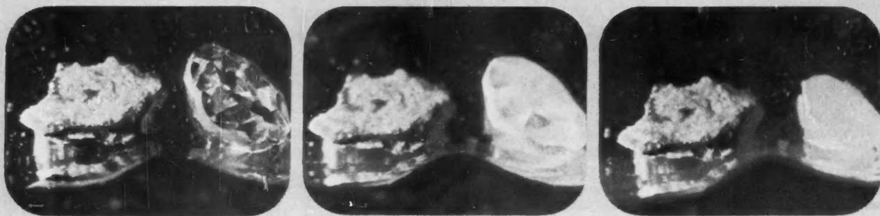
**BORAZON UNAFFECTED AS DIAMOND BURNS:** Picture sequence, taken at 30-second intervals, shows how a small gem placed on a resist-
