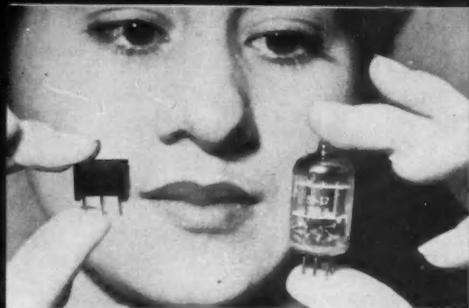
**MIDGET** double-diode selenium rectifier offers sizable savings to TV set manufacturers.
