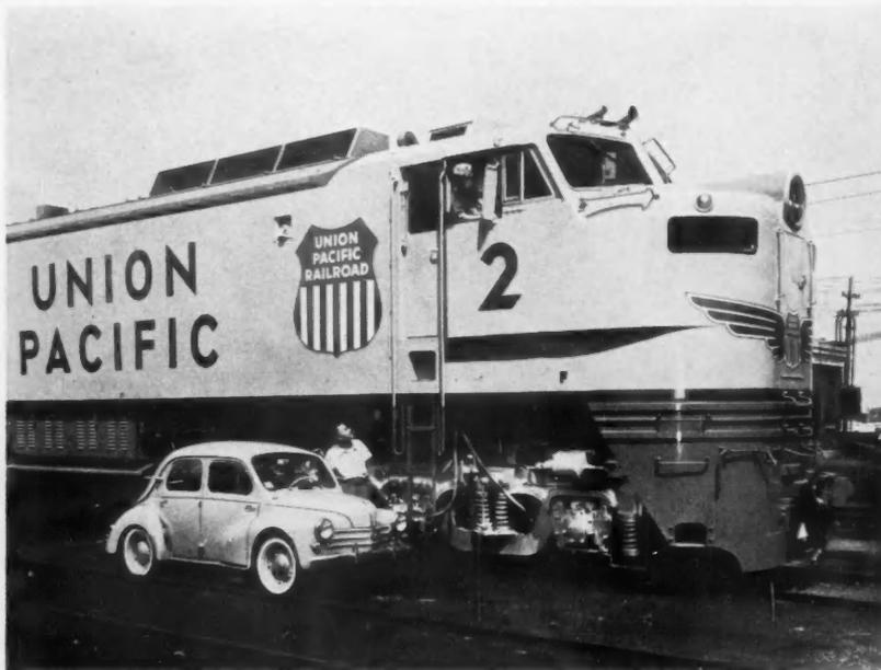
**HIGHER FREIGHT-TRAIN SPEEDS** in the mountainous terrain of the West will be met by 30 new 8500-hp gas-turbine electric locomotives being constructed for the Union Pacific.
