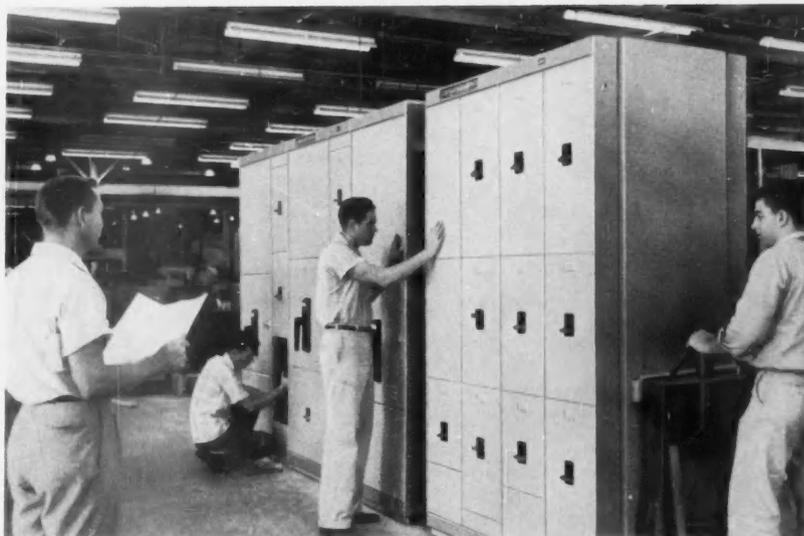
**LOW-VOLTAGE SWITCHBOARD** designed for incoming service to 600 volts was built in standardized modules for application versatility; main feeders are rated 800 to 4000 amp.
