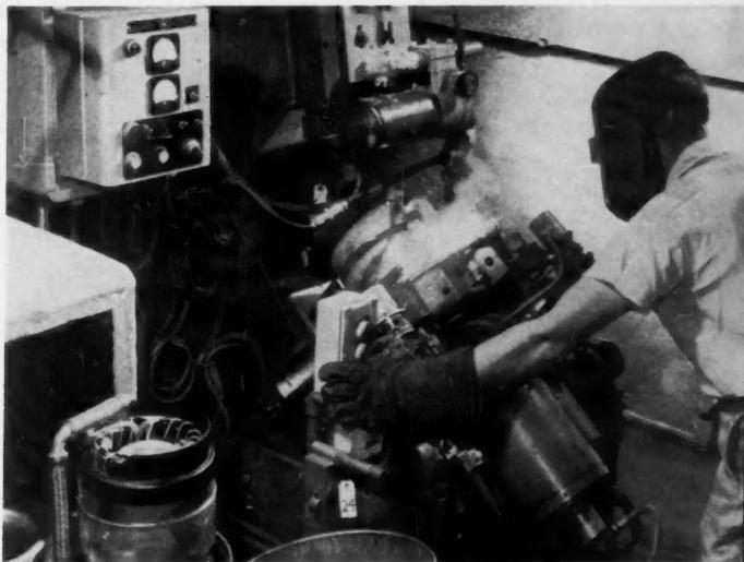
**HERMETIC SEALING** of compressors for new air-conditioners is carefully checked to provide air-tight operation throughout the life of the units.
