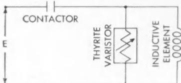
FIGURE 2 — Thyrite varistor surge voltage suppression circuit
