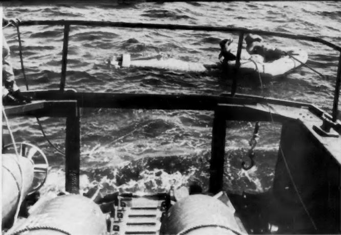
**3** Attaching the nose cage, a heavy steel towing device resembling a bottomless bird cage, is an exasperating, cold, wet job.
