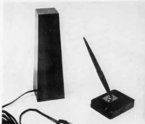
**SEPARATE TRANSMITTER** insures proper synchronization of electronic clock where normal 60-cycle field is insufficient.
