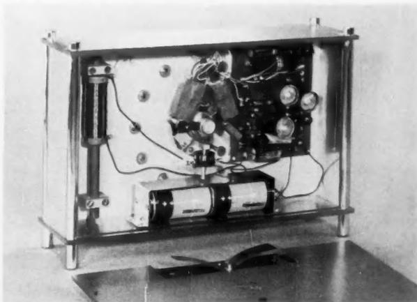
**MERCURY CELLS** power clock's miniature micropower motor for 18 months; ferrite antenna picks up the synchronizing signal.
