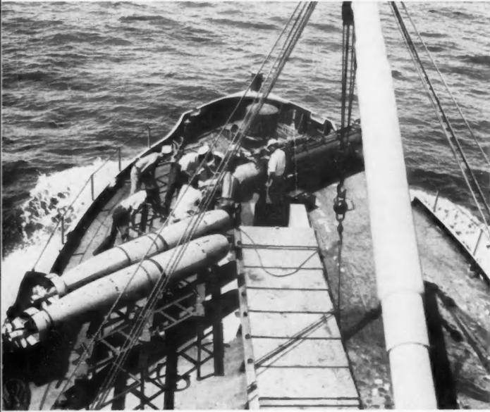
The activity prior to launching the acoustic homing torpedo begins the last and probably most critical phase of its development—tests in the sea.
