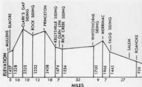
**PROFILE** of 134-mile electrified section from Roanoke to Mullens shows the steep grades. Climax is Clark's Gap: elevation 2525 feet.
