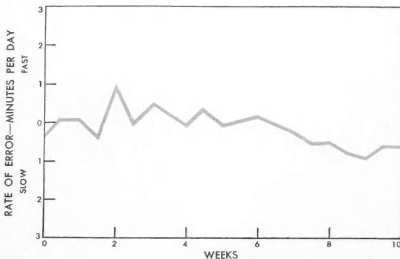
**TIMEKEEPING ACCURACY** during power failure is kept to within one tenth of a cycle by signal from clock's oscillator. Resetting is not needed even if power fails for several hours.
