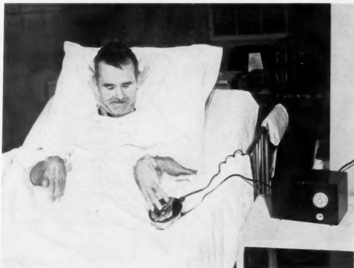
**KID BOZO**, former featherweight boxer, now a quadriplegic in Hillside Hospital, Bridgeport, Conn., has lost the use of his extremities because of a damaged spinal cord. But he can move his hand slightly to contact a touch-control unit, which turns on his radio. With the multiple touch-control unit (right), handicapped persons can control five different operations from a unit the size of a shoebox.
