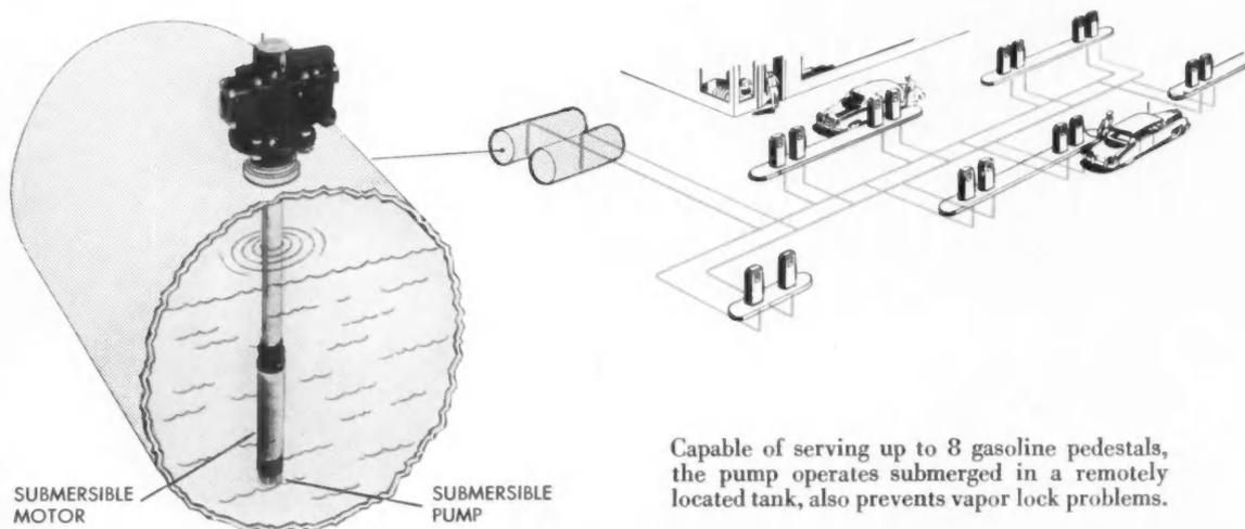
Capable of serving up to 8 gasoline pedestals, the pump operates submerged in a remotely located tank, also prevents vapor lock problems.
