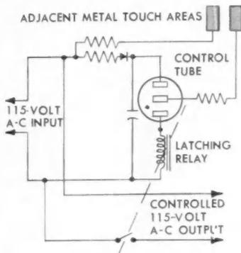
the portion of the hand bridging the touch area elevates the control-grid voltage. Impedance internally connected in series with each touch area limits this current, in microamperes, to well below the threshold point of sensation. Any external impedance, however, serves only to further desensitize the operation of the control.
