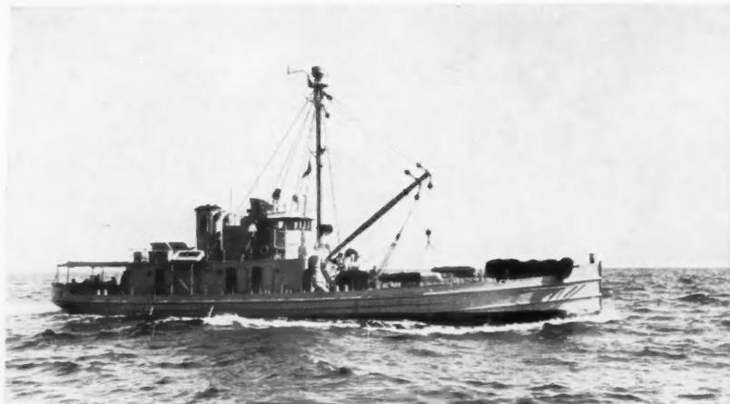
**YF** A converted yard freighter, it is equipped to launch torpedoes both from the deck and underwater. The deck launching tube, in the bow, is under wraps.
