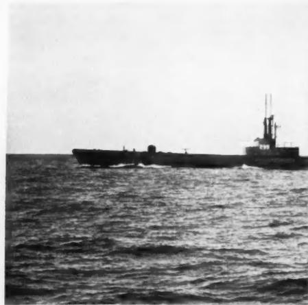
**TARGET** The submarine *Manta* has additional steel plate and a false hull
