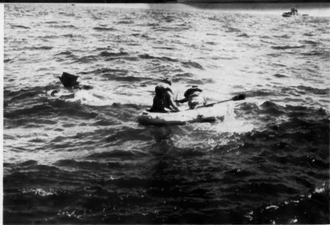
**2** Low buoyancy makes the torpedo (arrow) difficult to locate, but a vivid green dye helps by marking its position in the water.
