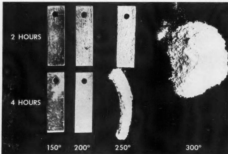
**CATASTROPHIC CORROSION** of aluminum in 300°C water is impeded by minor amounts of alloying nickel, which aids resistance by oxide-film modification.
