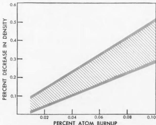
**UNALLOYED URANIUM** that is irradiated at low temperatures undergoes a decrease in density linear with exposure.
