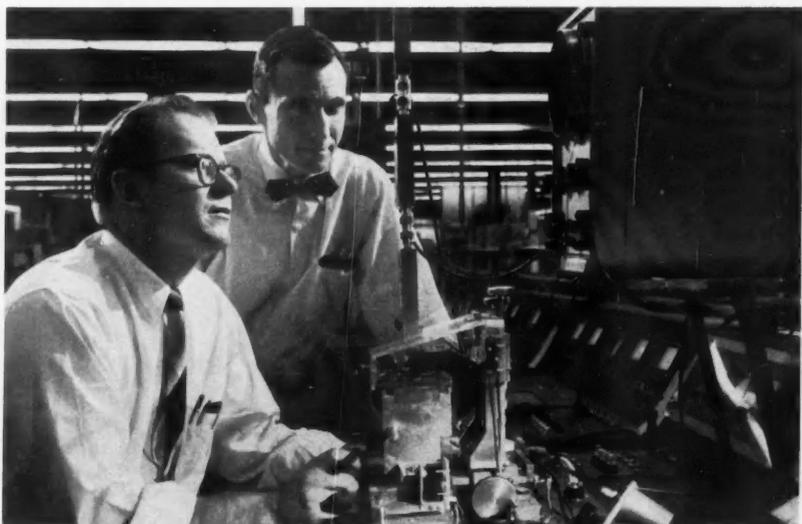
**WIDE-BAND SPECTRUM TESTS** from 2500–4000 megacycles are run on production voltage-tunable magnetrons by G. J. Griffin, Jr. (standing) and Frank Yatsko.
