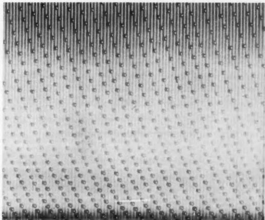
**MODEL** "electrons," constantly accelerating, roll down from cathode to anode. The visible electron tracks represent 90 exposures over a period of 1 1/2 seconds.
