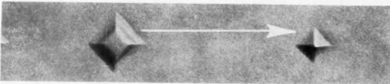
**MOTION OF DISLOCATION** is revealed in an actual crystal by flat-bottomed pit (left) at initial position and by sharp pit at position of dislocation after stress has moved it.
