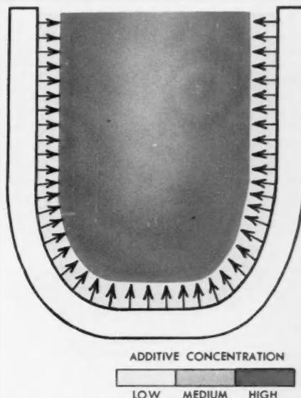
**COLUMNAR GRAINS** form at mold wall, grow inward. Additive rejected from growing crystals accumulates near interface and depresses the freezing temperature there.
