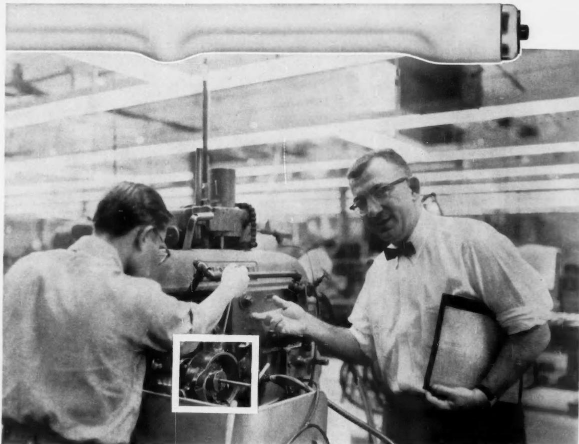
**SHADOW-FREE** lighting is pointed out by Mr. Steiner, standing at a milling machine. Notice, in the outlined area, the complete absence of shadows even inside the housing of the indexer.
