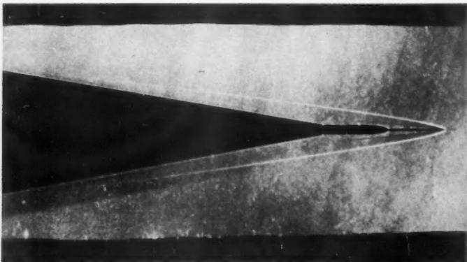
**RAZOR BLADE** is held in helium stream at Mach 22. The white line represents shock wave; the dark inside line marks the boundary layer.
