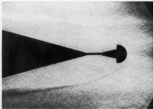
**HELIUM FLOW** forms shock-wave pattern around a 1/2-inch hemispherical model in tunnel at Mach 28.
