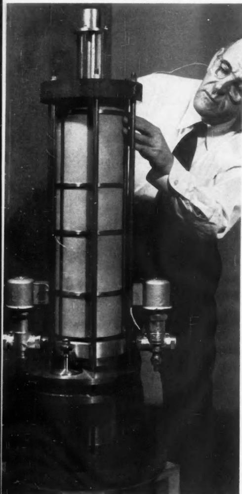
**MECHANICAL SWITCH** developed by Dr. W. F. Westendorp is used in large-scale plasma experiments; it can accurately control power in the order of 1000 megawatts.
