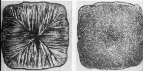
By inoculating a casting with special additives, scientists in the Research Laboratory have produced stainless steel with greatly refined grain structure (above, right) compared with characteristic columnar grain. This technique, although still experimental, resulted from a better basic understanding of how metals freeze from the melt. With E. Van Patten (center) are metallurgists James L. Walker (left) and A. J. Kiesler.
