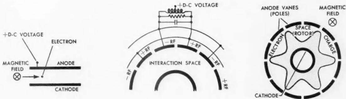
Electrons interact simultaneously with electric and magnetic fields oriented at right angles to each other (left). With the two forces effectively counteracting each other, the electrons move along the interaction space parallel to anode and cath-
