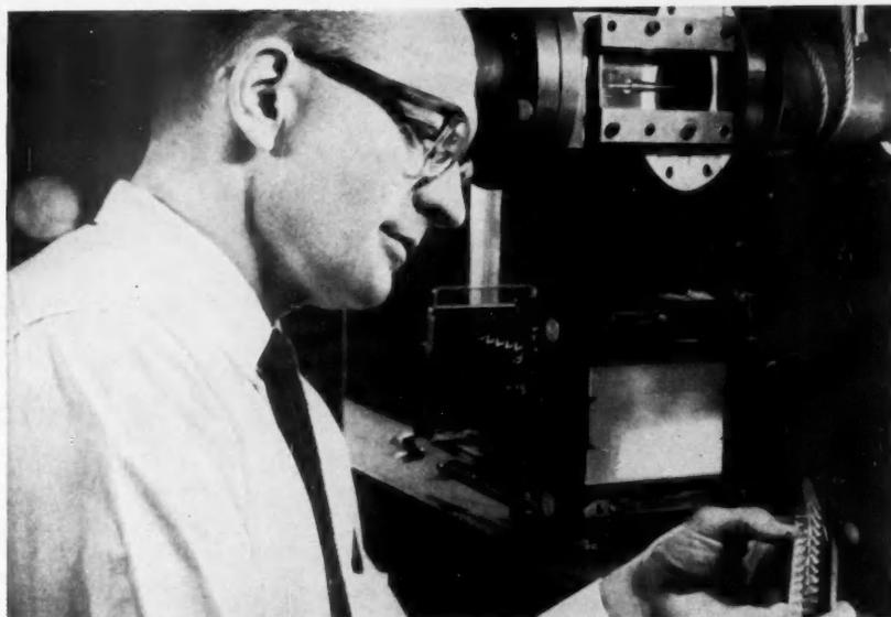
**CONE-SPHERE MODELS** used in experiments relating to the very-high-speed flight of missiles are examined. Model is visible inside tunnel's test section (above schlieren camera).
