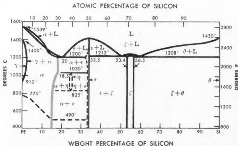
**SOLID SOLUBILITY** of silicon reaches 14 percent in alpha iron at 400 C (color curve). In spite of this, brittle behavior begins as low as 4 percent Si and persists up to 800-1000 C.
