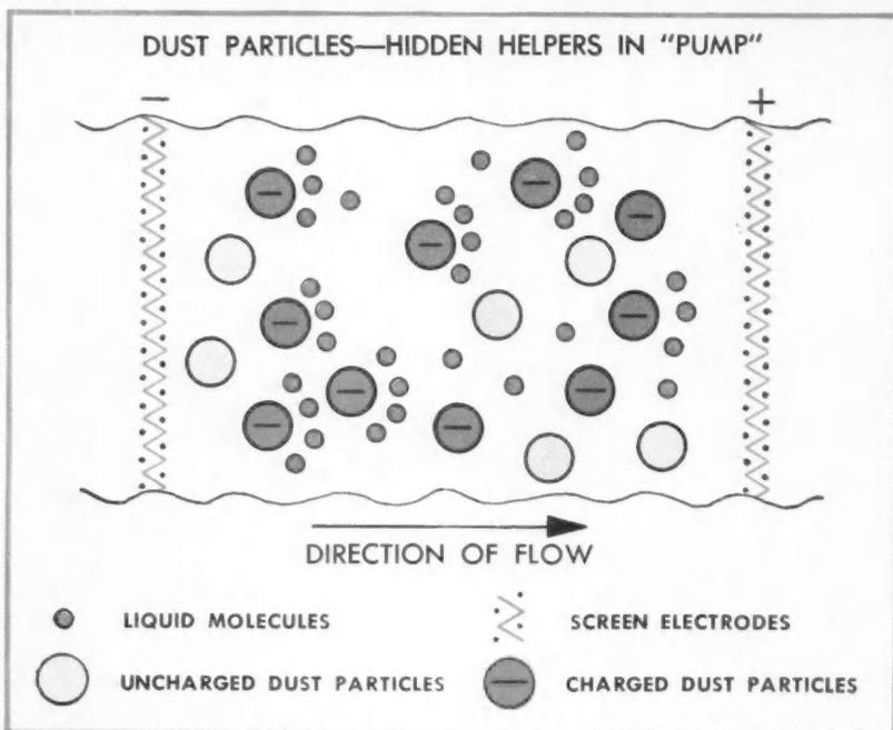
**CHARGED DUST PARTICLES** move toward anode. As dust collects out, pumping diminishes.
