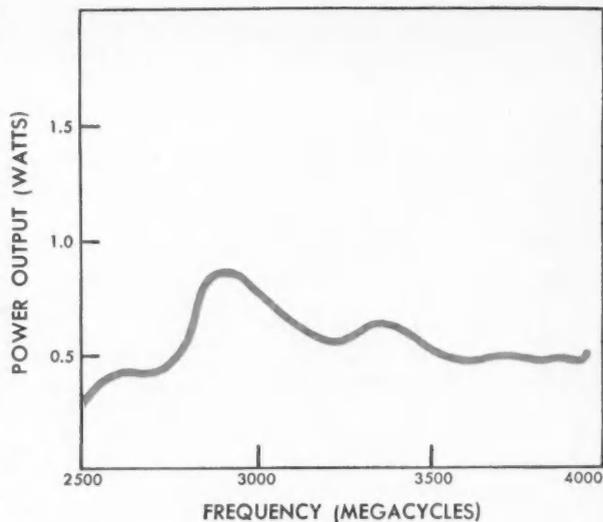
**FREQUENCY** set by the d-c anode voltage varies almost instantly. **POWER** up to 10 watts is possible through narrower tuning ranges.
