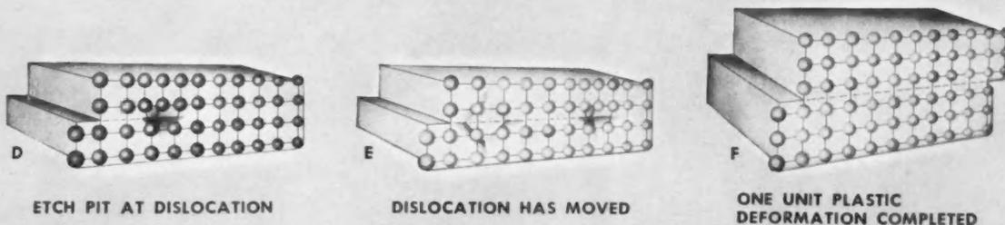
**DISLOCATION MOTION** inside a crystal permits plastic deformation. Acid easily attacks the crystal where the dislocation line intersects
