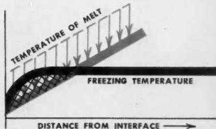
**AFTER INOCULATION** a supercooled region—represented by the crosshatched area—is formed, and new grains begin to freeze out ahead of the advancing interface.
