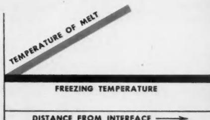
**PRIOR TO INOCULATION**, or in the usual situation, metal is at freezing temperature only at liquid-solid interface; so columnar grains grow inward from mold walls.
