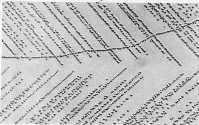
**PLASTICALLY BENT CRYSTAL** is etched in acid; one area (color inset) magnified 600 X (below) discloses long lines of etch pits that occur only in plastically deformed portion.
