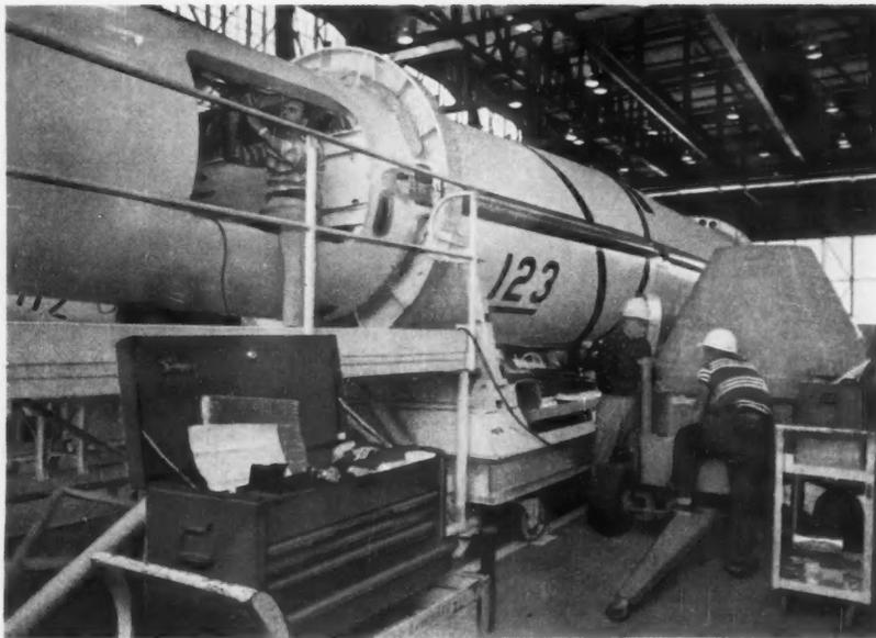
**Re-entry Vehicle** With electronic equipment to relay information back to earth during flight, re-entry vehicle (in orange handling dolly) will be installed on intermediate-range *Thor* missile.
