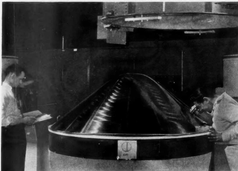
**Nose Cone** Polished to enhance the aerodynamic flow, the re-entry vehicle's conical shield (resting on a temporary base) undergoes "pit-plotting" inspection with optical enlarger that measures any minor surface defects.
