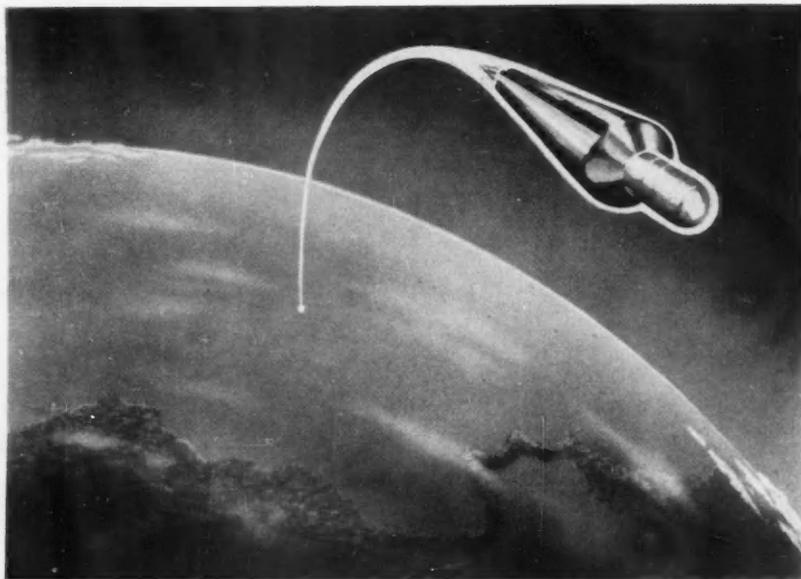
**Polaris Missile** Submarine-launched 1500-mile Navy weapon is aimed by computers correcting for the earth's rotation, wind, and vessel motion; guidance should be immune to electronic countermeasures.
