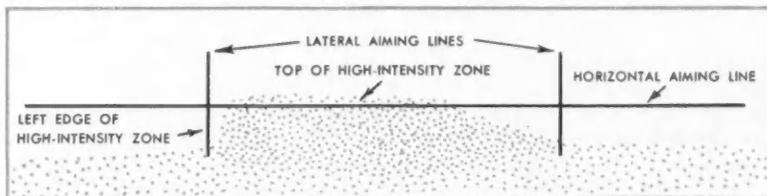
**SHADED AREA** (top) locates upper-beam aim for 7- and 5 $\frac{3}{4}$ -inch lamps and lower-beam aim (lower) for Type 2 (5 $\frac{3}{4}$ -inch) lamps and Suburban headlights, both with left lamp.
