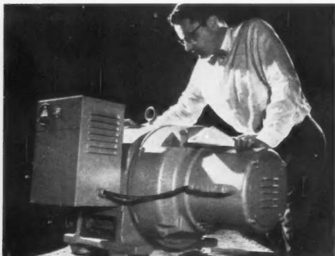
**BRUSHLESS A-C GENERATOR**, a 60-cycle machine with outputs of 40 to 150 kw, finds use wherever you need a reliable source of power—on farms, in industry, even for traveling road shows. In this generator, six hermetically sealed silicon rectifiers replace a multitude of brush and commutator parts that were subject to wearing and frequent adjustment.
