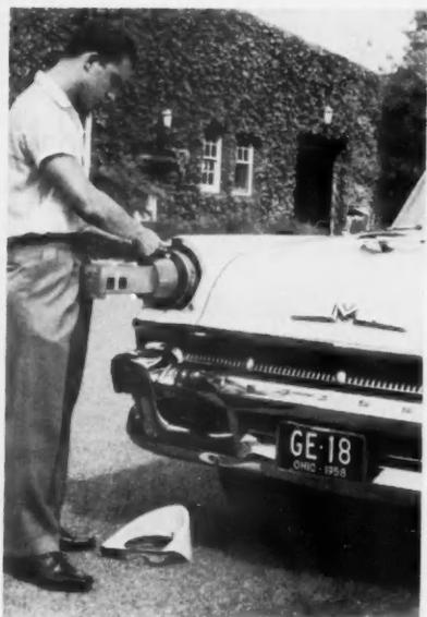
**AIMING HEADLIGHTS** is simple and exact with new mechanical device.
