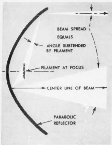
**BEAM DIVERGENCE** from any reflector point varies as the source size and reflector focal point.
