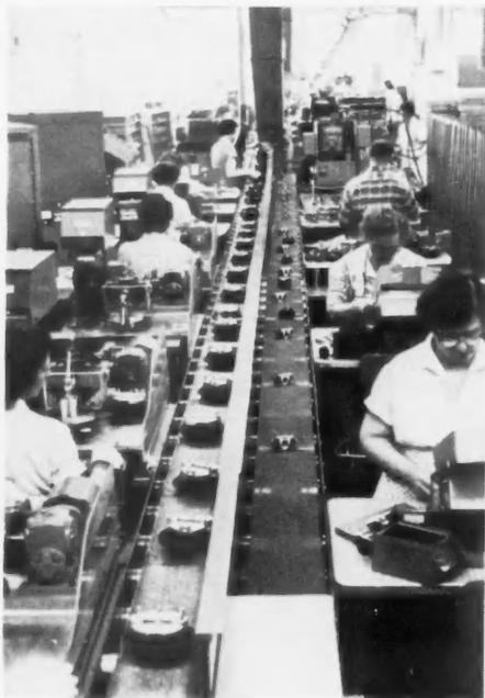
To minimize the manual handling of components, manufacturing engineers have applied mechanization to the assembly of watt-hour meters wherever feasible.
