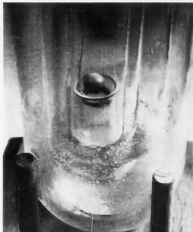
**MAGNETIC REPULSION** of superconducting metal ball supports it above toroidal magnet.
