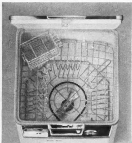
The new portable dishwasher has a stainless-steel impeller that drives wash water up through the dishes; reversed, it "pulls" the water down, forcing it out the drain. In addition, the sharp leading edge of the impeller chops up soft chunks of food soil for easy disposal.
