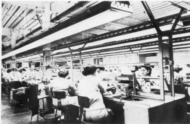
**LOCATING LIGHTING FIXTURES** five feet above work area at a Douglas Aircraft plant greatly cut wiring errors and improved employee morale by reducing tension and eyestrain.
