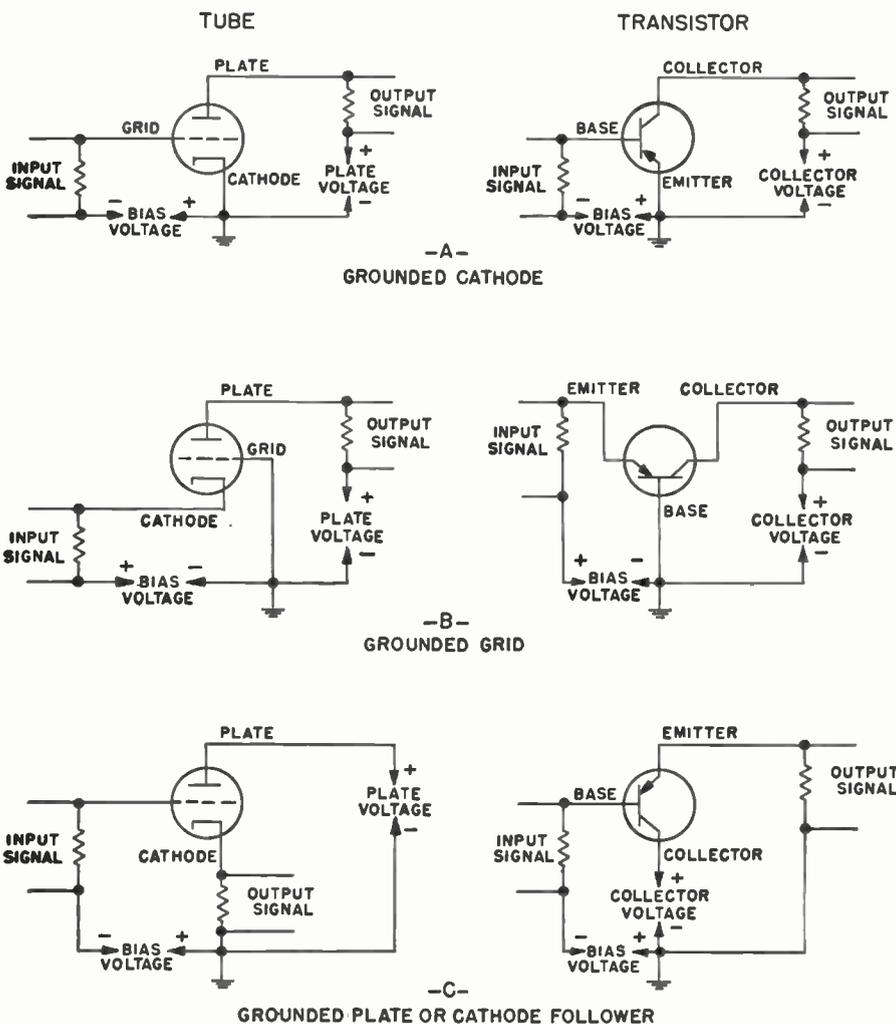
Fig. 5. Three typical tube circuits with comparable transistor circuits.
