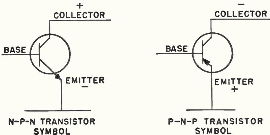
Fig. 2. N-P-N and P-N-P transistor symbols.
