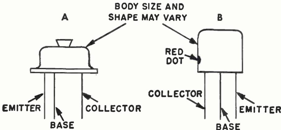
Fig. 4. Transistor basing and placement of leads.
