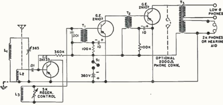
FIG. 6C. THREE TRANSISTOR BROADCAST RADIO
