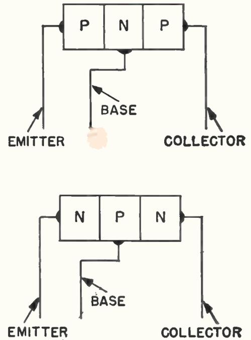
Fig. 3. Arrangement of elements in junction type transistors.
