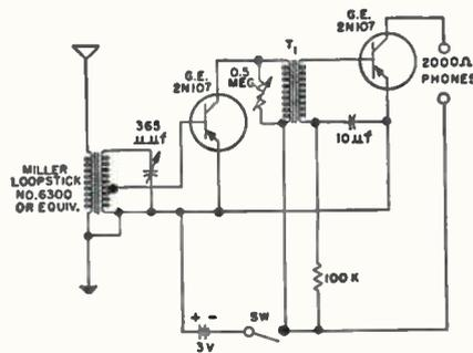
FIG. 6B. TWO TRANSISTOR RADIO RECEIVER
