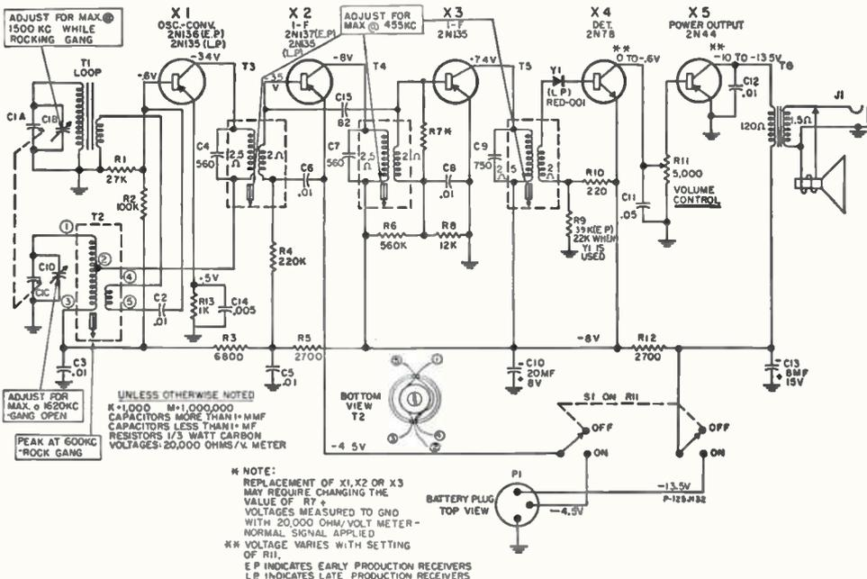
Fig. 7. Schematic diagram of General Electric transistor radio models 675 and 676.
