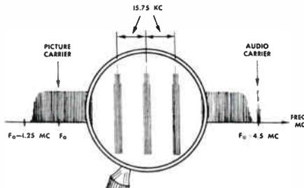
Fig. 12—Sideband spacing in monochrome channel.
