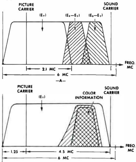
Fig. 11—Two methods of sharing 6 mc band.
