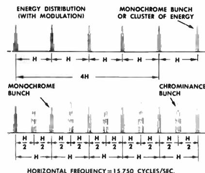
Fig. 13—Interleaving of brightness signal and chroma signal using sideband spacing effect.
