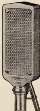
The newest development from the Brush laboratories in microphones for remote service. Built in a light but rugged aluminum case and being of the cell type it offers fine frequency response that is only possible with a cell type microphone. The B2S is not a diaphragm type microphone but a genuine broadcast device. Its response from 40 to 5000 cycles is flat and then rises about 6 Db. to 9000 cycles. The B2S will add crispness to your remotes and goes nicely with the
