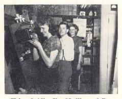
Helen Spidle, Jim Medlin and Dorothy Smyser are shown mounting subassemblies on panels to be installed in a BC1-F transmitter.
