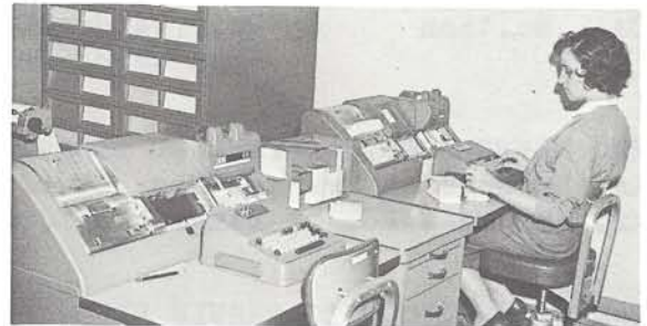
Here is Mary Bradley, key punch operator. Mary has punched thousands of cards to get our IBM system "on the road." She takes the original document and transcribes the information to obtain the punched card. This work is exacting for one error will throw off an entire report.
