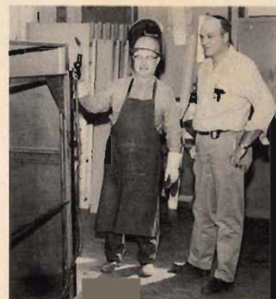
Dexter Wheelock, with the hood, and supervisor Royllyn "Bud" Wilson are shown with arc welding equipment. Arc welding adds metal to metal—filling openings that connect pieces of steel at corners, between cracks, etc., to form a solid unit.
