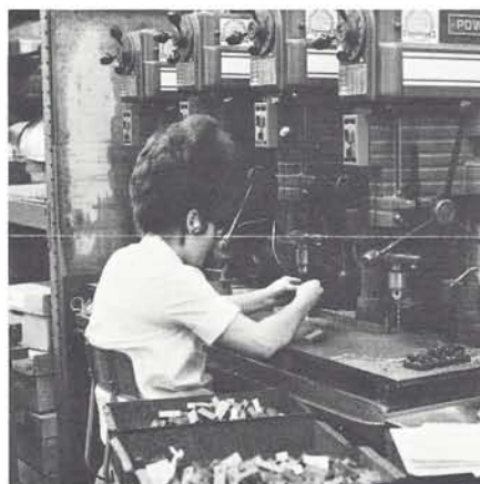
Linda Hendricks is operating the four spindle drills which are more efficient in that tool change time is reduced or eliminated. Handling time is improved over the single spindle machine that was formerly used.
