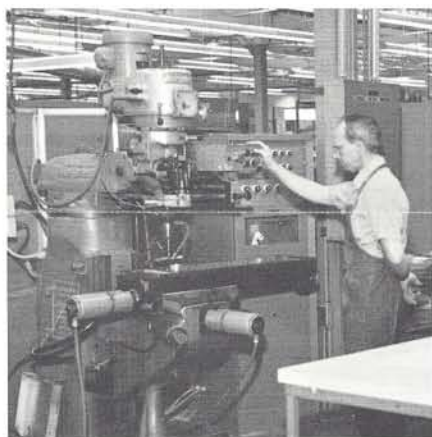
This automated machine center will reduce the cost of parts requiring milling or drilling and will permit more economical manufacture of Criterion 80 parts that have been previously purchased. Leo Clow is shown at the milling section of this machine center.
