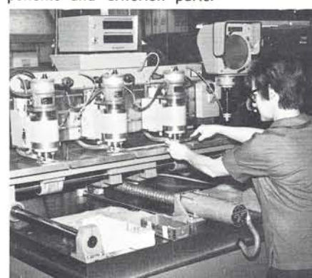
Pat Belker is shown performing a set-up and adjustment on the new Slo-syn N/C drilling machine which has been added to our new P.C. Board Facility. This new unit is self contained and can be used to produce N/C tapes from artwork as well as the actual drilling of printed circuit boards.
