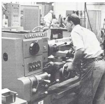
The Cincinnati Hydrashift lathe being operated by Luther Patrick is a high quality precision engine machine, capable of the close tolerance work needed in the production of TV components and 16" turntable platters.
