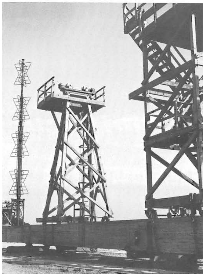
Harris TV antenna on test at the new range. Main turntable (foreground) is used in measuring horizontal and vertical patterns of larger Harris antennas.
