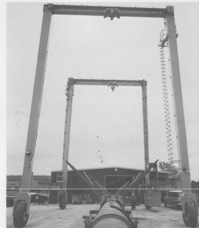
Here, the KTVI-TV antenna has been moved outside the manufacturing building (background) immediately after assembly, and is ready for the Travelift to carry it to the turntable area.
