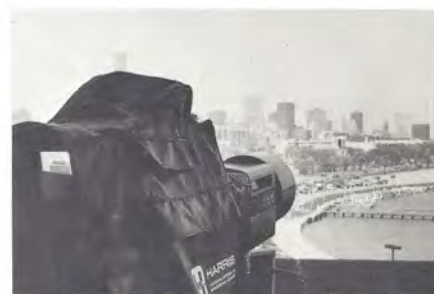
For the first time at a NAB Convention in the United States, a color camera...the Harris TC-80...was placed outside the equipment display. Operating with triax, it had a mile of cable between the camera head and the CCU. This picture shows the TC-80 on top of the McCormick building looking north along Chicago's Lake Michigan shoreline. Note the Hancock building as seen by the camera.
