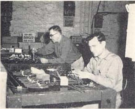
Larry "The Chief" Poor and Ed Lowary are wiring control panels as a sub-assembly operation.
