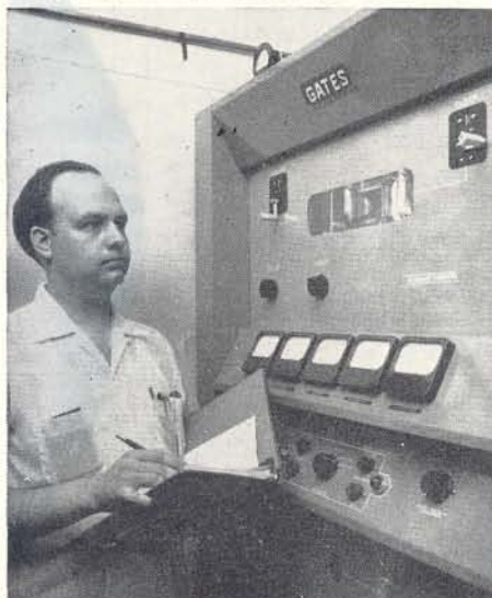
Pictured above is E. Harold Munn, Jr., Vice-President in charge of Engineering for the Christian Broadcasting Association. He is shown checking the operation of their Gates 1,000-watt transmitter. This installation incidentally is the first Gates AM broadcast transmitter in the Hawaiian Islands and we are very proud to have it at KAIM, one of Hawaii's most progressive stations.
