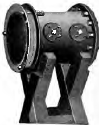
Fig. 2. Iron Cylinder Protected by Double Wire Gauze
