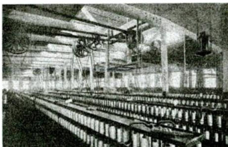
Fig. 4. Group of Spinning Frames in Cabarrus Mill, Driven by Motor Located Overhead
