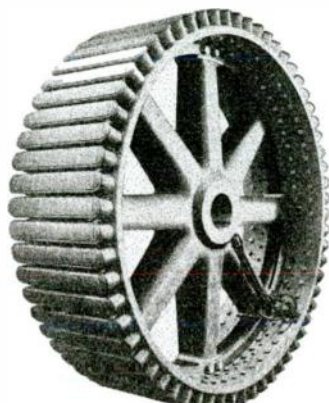
Fig. 2. Revolving field of 4000 kw., 116 r.p.m. three-phase generator, showing design generally used for moderate and slow speed generator; all castings are made to be free from shrinkage strains
