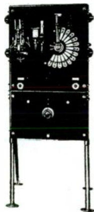
Fig. 1. Hand-operated Dial Controller used with direct current single motor semi-automatic printing press equipments. Push button jog; push button stop; no-voltage release; overload release; dynamic brake; slow speed; armature and shunt field regulation are provided.
