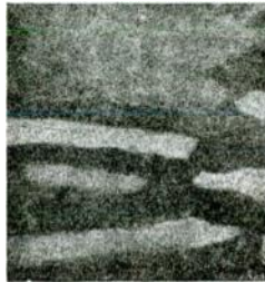
Fig. 1. Structure of Cast Copper Just Beyond Original End of Bar
