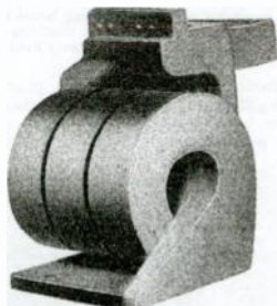
Fig. 6. Blow-out Coil Cast in One Piece by the Use of Boron Suboxide. Turns Squeezed Together After Casting
