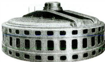
Fig. 6. 2500 kw., 97 r.p.m. three-phase generator, showing the appearance of a slow speed machine with the top bracket provided with a bearing for supporting the weight of the revolving part of the generator and the waterwheel runner
