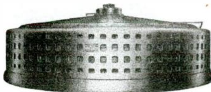
Fig. 1. 9000 kw. 57.7 r.p.m., 11,000 volts, three-phase generator, showing general appearance of a very slow-running large size generator
