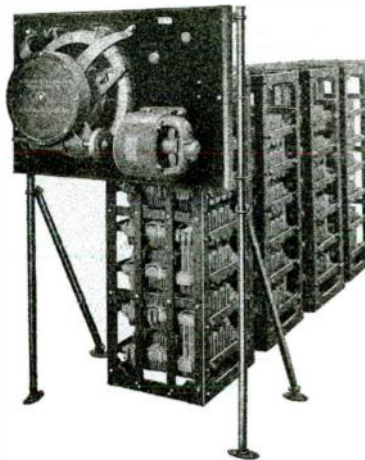
Fig. 8. Motor-operated Field Rheostat for 14,000 Kw. Turbo-alternator
