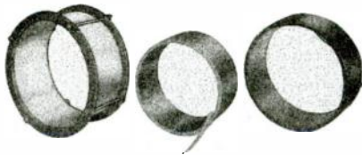
Fig. 2. Coils and Clamping Ring of Constant Current Transformer
