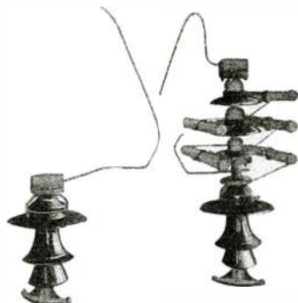
Fig. 1. One Form of Mounting Charging Resistance for the Aluminum Arrester
