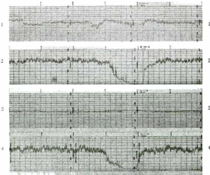
Fig. 36. The effect of automatic power-factor correction is illustrated by the above voltage curves taken at Rome. Curve No. 1 shows the voltage when controlled by a feeder regulator, but operated beyond its limit, and curve No. 2 the corresponding currents. Curve No. 3 shows the voltage regulation accomplished by a 1000 kv.-a. synchronous condenser with a voltage regulator. Curve No. 4 shows the corresponding currents. Though the currents in curves 2 and 4 are approximately the same, the energy delivered in the former case was during the day around 600 and 700 kw., while with the corrected power-factor in curves 3 and 4, the energy delivered was around 1000 kw. It is interesting to note that the power-factor remains around 1.00 from no-load to full load. This was shown in Fig. 18
