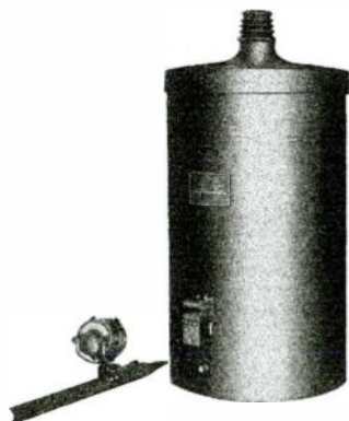
Fig. 2. Ammeter, Stick and Jack for Measuring the Charging Current in an Aluminum Arrester
