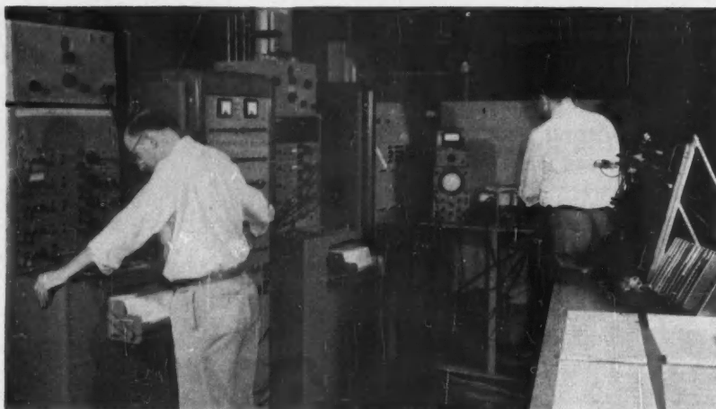
TRANSIENT RESPONSE of proposed control system for a jet engine is recorded in a matter of seconds by author Bradford (left) with an electronic analog computer.
