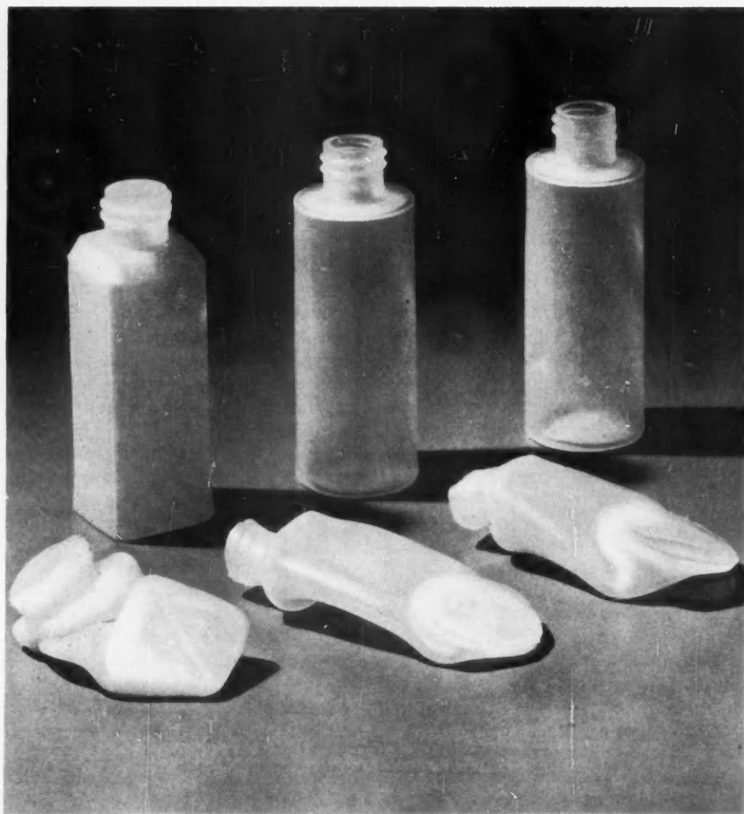
POLYETHYLENE BOTTLES melt at temperatures slightly above that of boiling water; if irradiated, they retain their shape even after being subjected to 250 F for 20 minutes.
