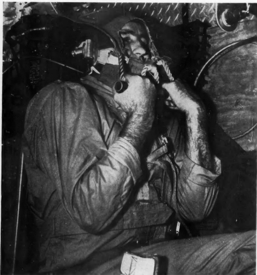
INSTRUMENTED for ejection-seat test run, chief engineer Howard Hunter yanks protecting windscreen down in front of his face. This would simultaneously eject the seat from an aircraft. Changes in blood supply to head are detected by photoelectric instrument.
