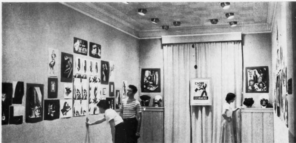
SPECIAL LIGHTING EFFECTS—IDEAL FOR ILLUMINATING EXHIBIT ROOMS—CAN BE OBTAINED BY USING SEMIRECESSED ADJUSTABLE SPOTLAMPS.
