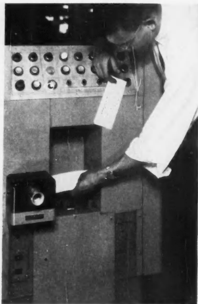
TURRET PUNCH PRESS , controlled by cards like those used in business machines, automatically punches predetermined holes in a sheet
