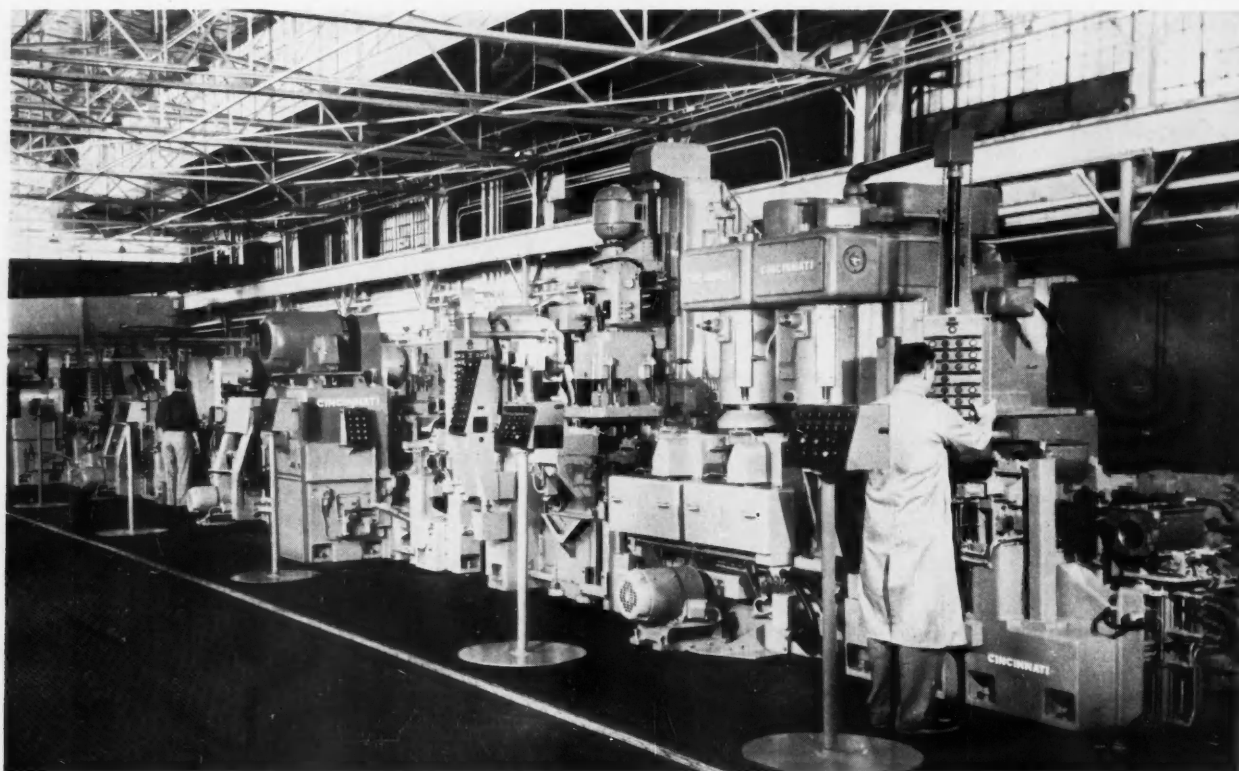
ELECTRIC CONTROLS MOVE WORK THROUGH 37 STATIONS IN TRANSFER MACHINE THAT MAKES AUTOMOBILE TRANSMISSION CASES.
