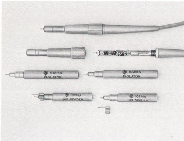
Fig. 10. Probes and accessories for *-hp-* Model 8405A Vector Voltmeter. Top to bottom: assembled probe; exploded view of probe, showing sampler circuit; isolators, 10:1 dividers, and ground clips supplied with probes. Isolators (or dividers) and ground clips are used when probing by hand in arbitrary circuits. (Tees and adapters are available for probing in 50-ohm coaxial systems.) Dividers extend upper limit of voltmeter range to 10 V. See Specifications for details.
