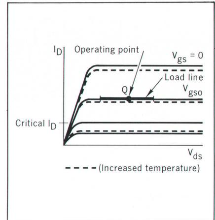
Fig. 4. Typical characteristic curves for field-effect transistor. Increase in temperature changes  $V_{GSO}$  of load line to compensate for temperature-induced changes of operating points in associated bi-polar transistors.
