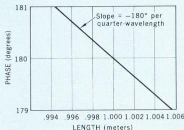
Phase versus length of cable for system shown in block diagram, calibrated at 75 MHz (quarter-wavelength = 1 m). Phase resolution of VVM is  $0.1^\circ$ , allowing length to be determined within 0.6 mm at 75 MHz, or more accurately at higher frequencies.
