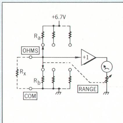
Fig. 8. Ohmmeter circuits.
