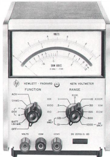
Fig. 2. —hp— Model 427A Voltmeter measures ac volts from 10 mV to 300 volts full scale, resistance in 7 ranges from 10 ohms to 10 megohms center scale, and dc volts from  $\pm 100$  mV to  $\pm 1000$  V full scale. Input impedance is 10 megohms in both ac and dc voltage-measuring modes.
