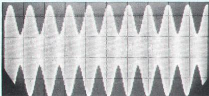
20-kHz IF output of Vector Voltmeter observed on *hp-120B* Oscilloscope (bandwidth = 450 kHz). Input to VVM was 300-MHz carrier, amplitude modulated by 1-kHz signal. Oscilloscope was synchronized to modulating signal only.
