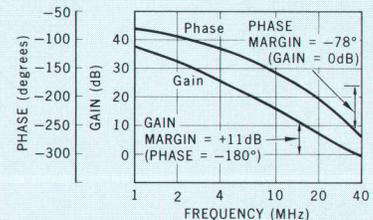
Open-loop gain and phase shift for a transistor amplifier circuit as measured with RF Vector Voltmeter. Amplifier was unstable, as gain and phase margins indicate.
