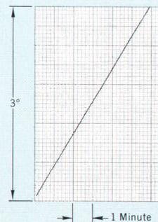
scale is 12 seconds per division, and the full-scale phase difference is  $3^\circ$ . The slope of the trace can be determined within less than one minute, whereas older methods would have required much longer to achieve this precision.
