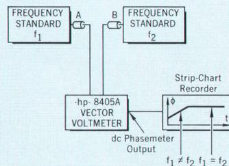
If the frequencies of the two oscillators are the same their phase difference will be constant. If the frequencies differ, the phasemeter reading will change at a rate given by
