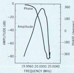
Gain and phase shift of *hp*- Model 8442A 20-MHz Crystal Filter as measured with new RF Vector Voltmeter.
