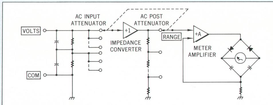
amplifier that matches the input to the low impedance of the meter movement, using the FET to achieve very high input impedance.
