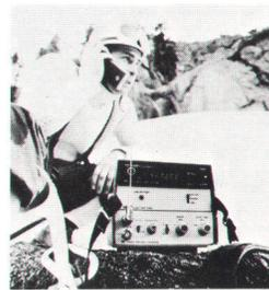
**Cover:** You probably wouldn't find a 5300 Measuring System among a mountain rescue team's standard equipment. But one could be used at the base camp for checking vital radio equipment. Shown here is all it takes: a 5300A mainframe, a 5310A battery pack, a 5303A 500 MHz counter module, and a makeshift antenna.
