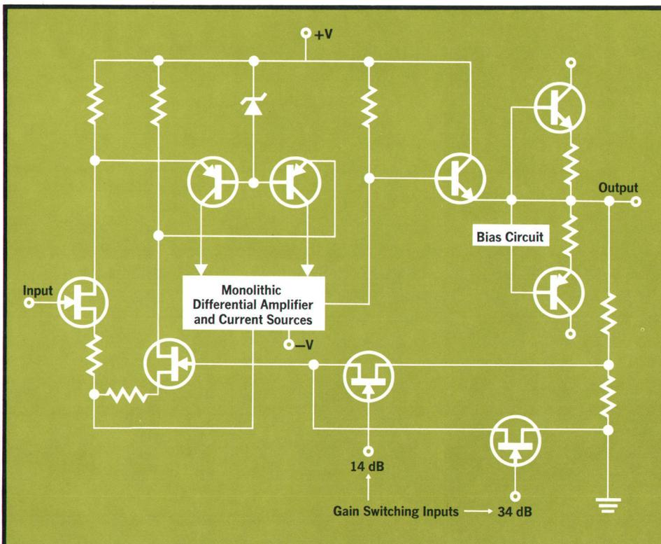
**Fig. 3.** Input amplifier simplified schematic. The 3403 input amplifier uses a combination of technologies. The substrate is ceramic with laser-trimmed thin-film resistors and conductors. Mounted on the substrate in chip form are JFET's, diodes, bipolar transistors, a high-frequency monolithic bipolar IC, MOS capacitors, and ceramic capacitors. Except for emitter-follower output drive the entire circuit is differential.
