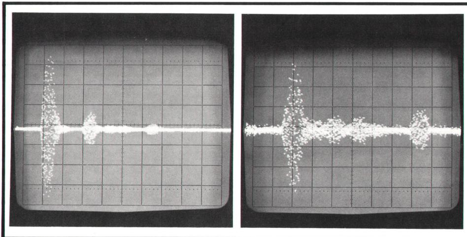
**Fig. 7.** Multiple discontinuities are separated on display for easy identification. Photo at far left, with horizontal scale of 10 ft/div, clearly shows discontinuities at 22 feet and 54 feet and it indicates possibility of discontinuities at 32 and 40 feet. Expanding horizontal scale 2 times and vertical scale 5 times (photo near left) shows that these suspected discontinuities do exist, that they have a reflection coefficient of 0.03, and that they are 7 feet apart.
