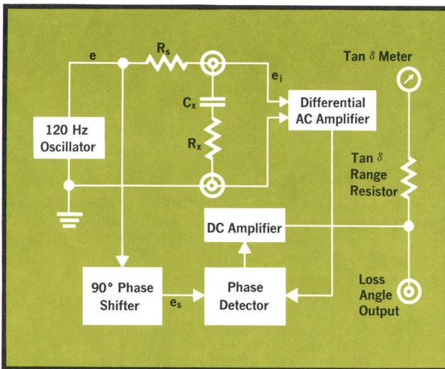
Fig. 8. Measuring circuit to determine dissipation factor.
