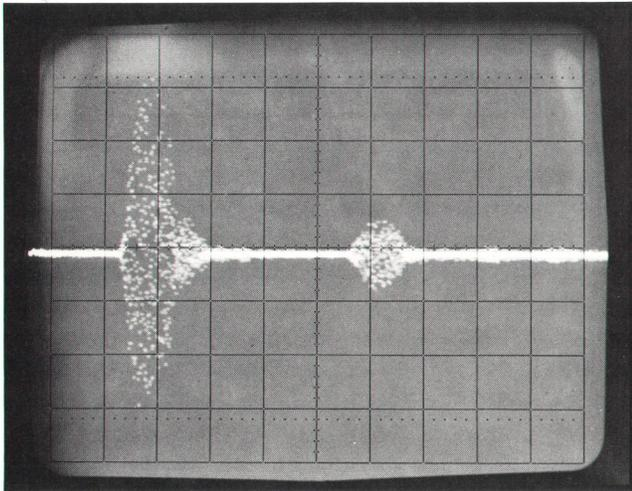
**Fig. 5.** Typical narrowband TDR display showing interrogating 10-ns burst of 6-GHz carrier and 20% reflection from impedance discontinuity. Horizontal scale factor of 10 ft/div establishes distance to discontinuity as 44 feet.
