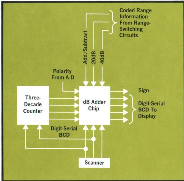
**Fig. 6.** Ranging of dB display. A single MOS chip, a serial adder, performs display ranging in the dB mode. Signals from range-switching circuits command the adder chip to add or subtract 20, 40 or 60 dB to or from the serial BCD generated by the A-D Converter of the digital panel meter.
