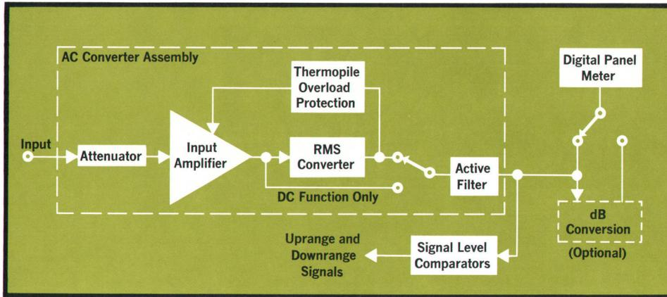
**Fig. 2.** The basic design of the 3403A is simple and straightforward. The performance of the instrument is largely due to the capabilities of the hardware used. Included are HP-built components using six different new technologies: 1) thin-film hybrid, 2) monolithic bipolar (conventional), 3) monolithic bipolar (high frequency), 4) MOS LSI monolithic, 5) thin-film vacuum thermopile, and 6) GaAsP light-emitting diodes.
