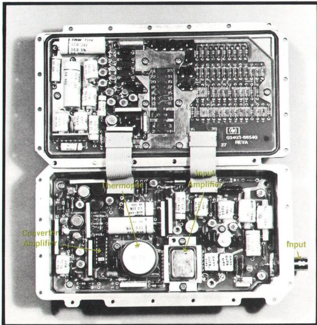
**Fig. 7.** AC converter assembly. Aluminum casting is hermetically sealed to prevent high-frequency humidity problems. Inside is the thin-film thermopile and the dc-to-100 MHz thin-film hybrid IC amplifier.
