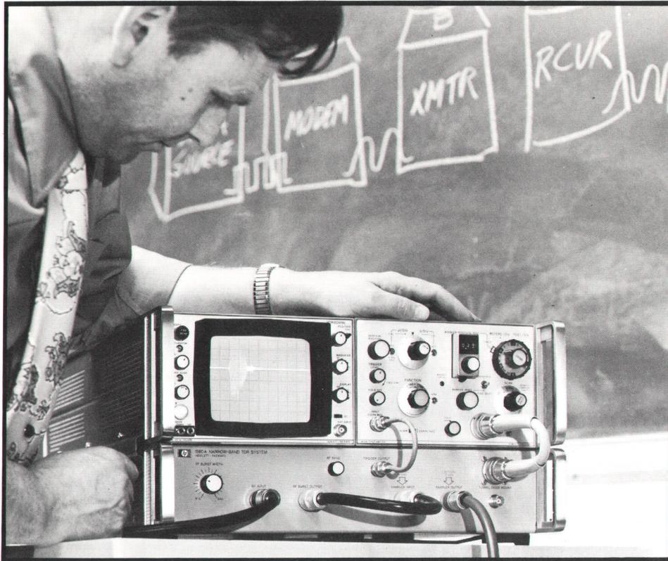
**Fig. 1.** Impedance discontinuities in waveguide and narrowband coaxial transmission systems are easily located with Model 1580A Narrowband Time Domain Reflectometer System. Microwave signal source (not shown) supplies energy for RF bursts. System can also be used for wideband applications with optional tunnel diode voltage step generator.
