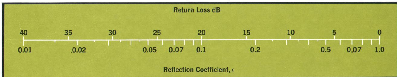
**Fig. 6.** Nomograph converts reflection coefficient into return loss.
