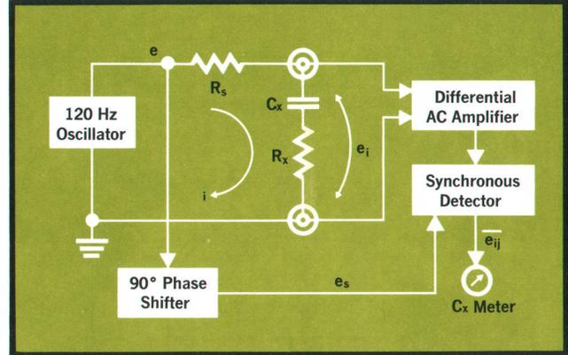
Fig. 5. Voltage-current method commonly used for capacitance measurements.
