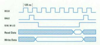
Fig. 3. A typical six-BCLK ISA cycle.
