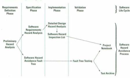
Fig. 6. Software hazard avoidance process flow in the software life cycle.
