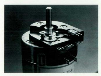
Fig. 1. Robot position encoder mounted on a servo motor
