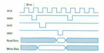
Fig. 5. Typical host bus cycle.
