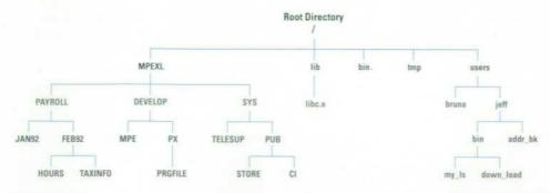
Fig. 5. A directory structure that was rejected for MPE/iX.
