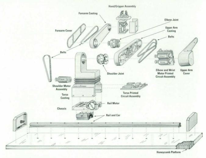
Fig. 3. Exploded view of the robot arm.
