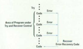
Fig. 3. The control flow for a try/recover statement.
