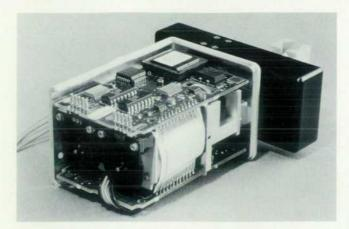
Fig. 4. Interior of robot hand.
