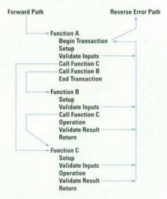
Fig. 2. Transaction error-handling program flow.
