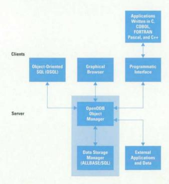
Fig. 2. HP OpenODB client/server components.
