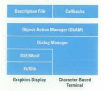
Fig. 1. The SAM user interface software architecture.
