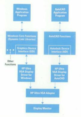
Fig. 11. Software hierarchy from the application to the display driver.
