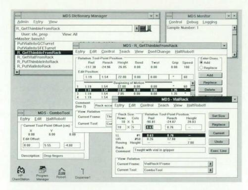
Fig. 9. Robot motion, rack, and tool editors.
