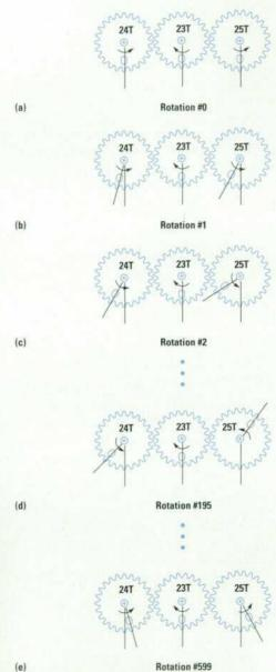
Fig. 2. Absolute digital encoder operation
