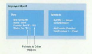
Fig. 3. The structure of a typical object. Notice that the data part contains pointers to the data (or other objects).
