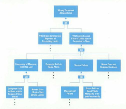
Fig. 3. An example of fault tree analysis.
