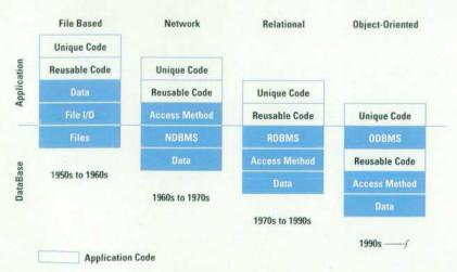
Fig. 1. With each new database architecture more and more major components have been moved from the application level to the database level. The years show approximately when the architecture was introduced and the peak years of use. By the way, all of these architectures are still in use.
