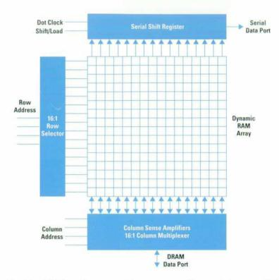
Fig. 7. Simplified diagram of a VRAM.
