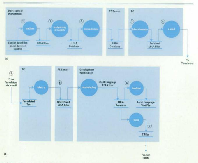
Fig. 2. The typical life cycle of a text file that is translated with the localization tools. (a) The flow from originating division to translators. (b) The return flow from translators to product ROMs.
