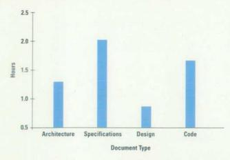
Fig. 5. Average hours per page by document. Each of these times includes preparation, defect logging, and rework time.
