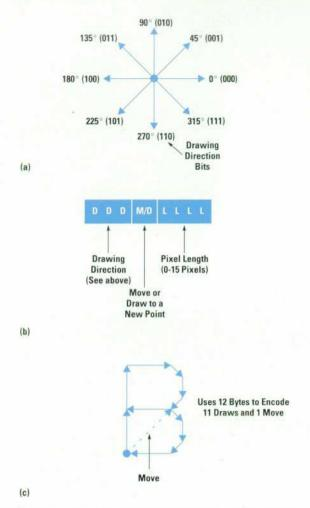
Fig. 2. (a) Short stroke vector directions. (b) Byte encoding of a short stroke vector. (c) Example of a character drawn using short stroke vectors. This character would require 48 bytes if stored as normal long vectors—12 X and 12 Y values each two bytes long.
