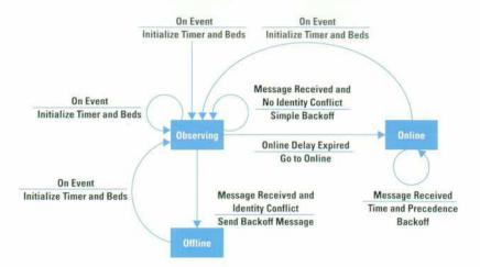
Fig. 5. An example of event tree analysis using a state machine approach. A backoff message tells the instrument to ignore any further messages or alarms.
