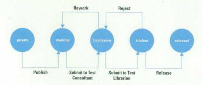
Fig. 5. The TLMS main life cycle. Test assemblies or individual component versions move through this life cycle.
