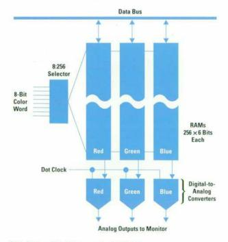
Fig. 8. Simplified diagram of a RAMDAC.
