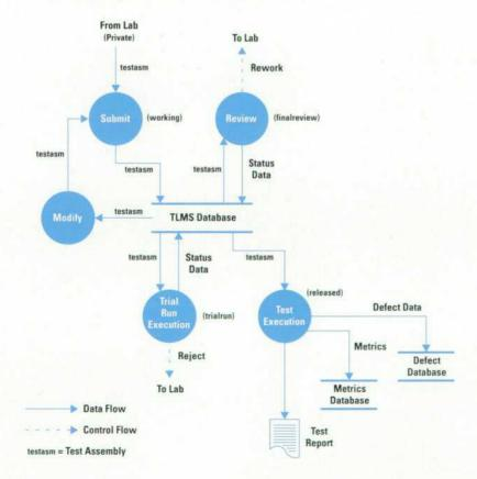
Fig. 7. The test process with TLMS in place. The items in parentheses are the states in the main TLMS life cycle shown in Fig. 5.
