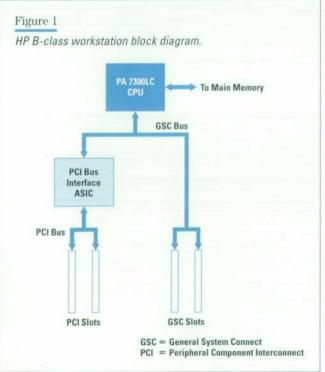
read data from the PCI bus back to the GSC bus. Since the read originates in the processor, this task is called a processor I/O read.
