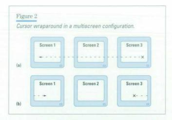
For example, on an HP 9000 Model 715 workstation containing an HCRX24 display (a 24-plane device) and an internal color graphics display (an 8-plane device), the user can still create a multiscreen configuration. Of course, those applications directed to the HCRX24 will have access to 24 planes while those contained on the other are limited to 8 planes. Currently, the HP-UX X server allows a maximum of four graphics devices to be used in a multiscreen configuration.
