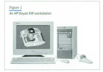
the performance available in the graphics hardware, the bus interface had to be changed from the standard Peripheral Component Interconnect (PCI) to the accelerated graphics port (AGP),† since no commodity PC chipset supported PCI 2X. With normal industry-standard PCI, we would have been limited to 132 Mbytes/s for I/O, which would have hurt our performance on several important benchmarks. With the accelerated graphics port, the available I/O bandwidth increased to 262 Mbytes/s.
