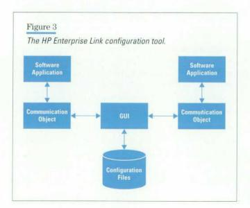
All dependencies on particular software applications are encapsulated in communication objects. The configuration tool's communication objects provide the following functionality:
