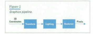
triangle strip, quadrilateral, or polygon. Based on the type and count, the vertices are assembled together as primitives and sent down the rendering pipeline.
