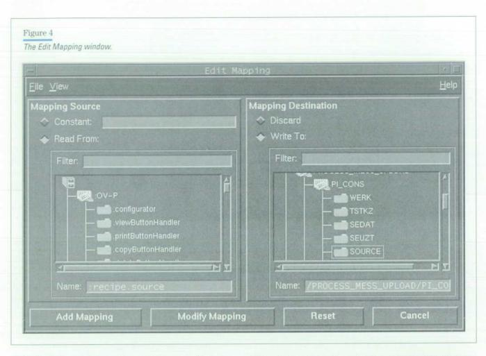
Multiple static mappings can be created in a single step using branch assignments. This requires that the last component of the source and destination addresses be identical (so that appropriate mappings can be automatically created). Mappings can also be automatically created at the time methods are triggered. This is called dynamic mapping and requires the user to specify algorithms that can select source addresses and transform these addresses to valid destination addresses.
