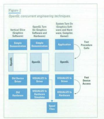
the pieces at the end. This would result in a longer and less predictable time to market. Instead, we created a prototyping environment. This environment was initially created to test the software architecture and early design decisions. The life cycle included a number of checkpoints focused on interface specification, design, and prototyping.
