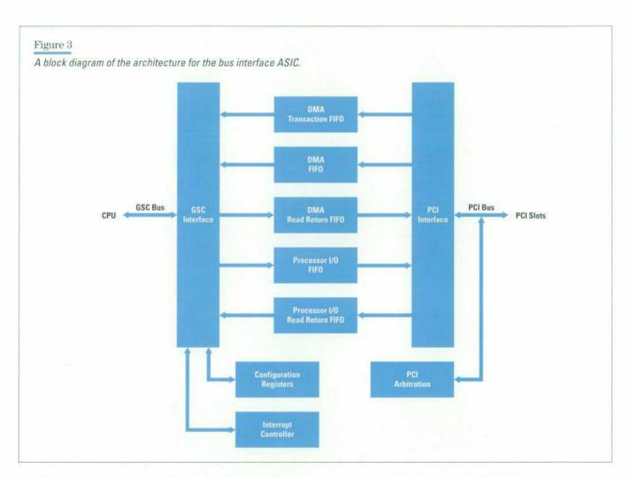
A FIFO is a memory device that has a port for writing data into the FIFO and a separate port for reading data out of the FIFO. Data is read from the FIFO in the same order that it was written into the FIFO. The GSC bus clock is asynchronous to the PCI bus clock. For this reason, the FIFOs need to be asynchronous. An asynchronous FIFO allows the data to be written into the FIFO with a clock that is asynchronous to the clock used to read data from the FIFO.
