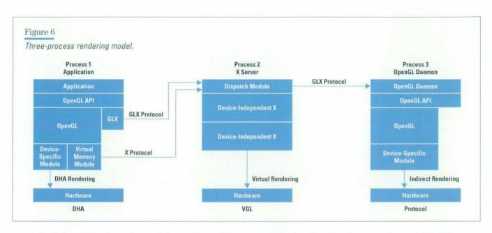
coupled with two distinct remote rendering modes, making our OpenGL implementation one of the most flexible implementations in the industry. These rendering modes are based upon the three-process rendering model shown in **Figure 6**. This model supports three rendering modes: direct, indirect, and virtual.
