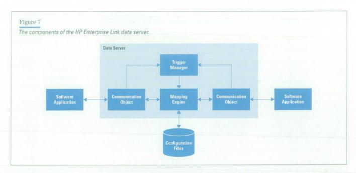
aware of its own namespace and how to convert between the software application's proprietary data formats and the neutral HP Enterprise Link data format. For triggers, the interface consists of well-documented interactions between the trigger manager and the communication objects.
