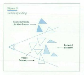
that can be rendered in the time allowed for the frame. Algorithms that perform this geometry reduction fall into two broad categories: *culling*, which eliminates unnecessary geometry, and *simplification*, which replaces some set of geometry with a simpler version.
