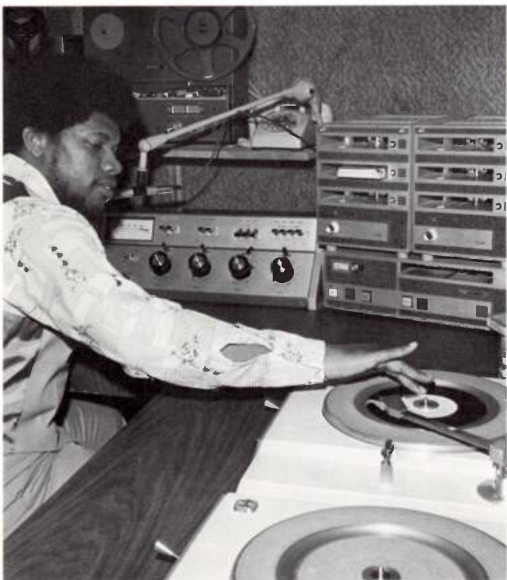
Ron Williams cues a record on a Harris CB-1201 Turntable. Both control rooms are almost entirely Harris equipped, including Dualux 80 and Stereo 80 audio consoles, four CB-1201 turntables and several Criterion cartridge machines.
