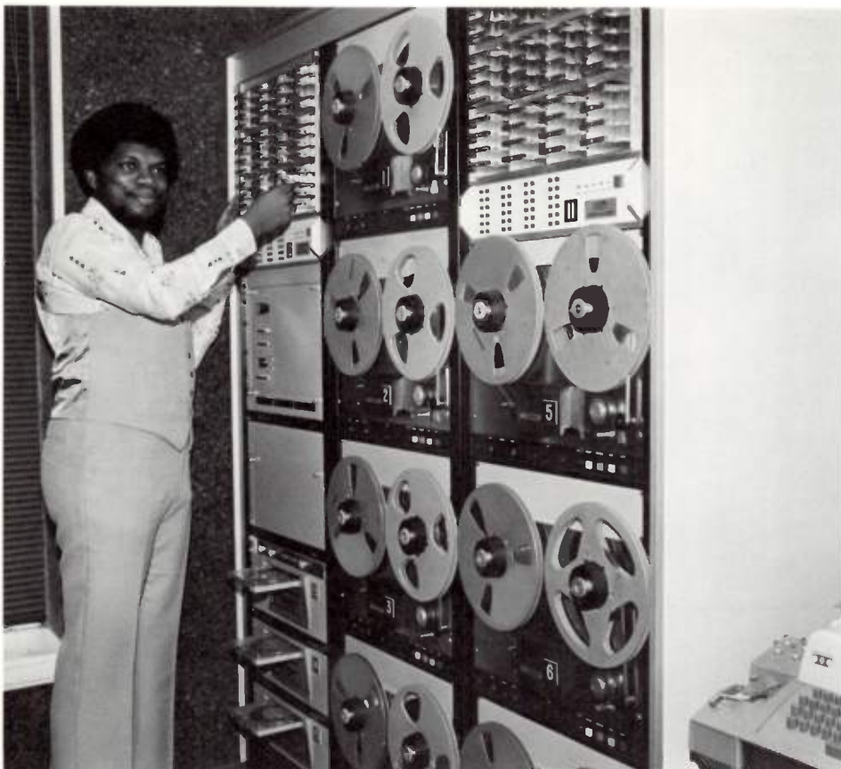
Program Manager Ron Williams pulls a cart from the new Harris System 90 program automation system which is used by KFJL-FM. A Teletype 33 ASR clear text logger is used with the System 90.
