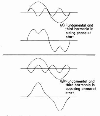
Fig. 7. Dependence of Wave Form on Phases of Components
