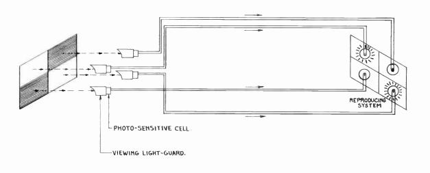
Fig. 2. Multi-Channel Transmission of Very Simple Changing Picture.
