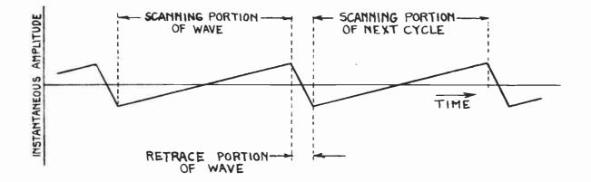
Fig. 6. Saw-Tooth Wave Form.
