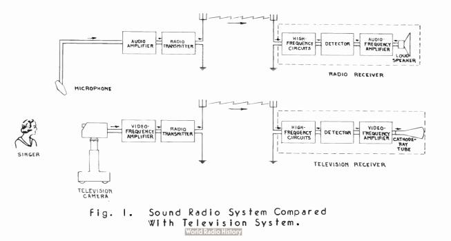
seen and it is unnecessary to describe the functions of these parts. Also at the sound receiver there are the high-frequency circuits, the detector, the audio amplifier, and the loudspeaker, which together constitute the radio receiver.
