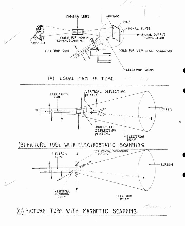
Fig. 5. Electronic Scanning Arrangements.
