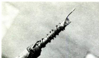
Figure 3. Excess heat from large irons can be reduced by technique shown. Number 10 or 12 gauge copper wire serves as soldering tip.
