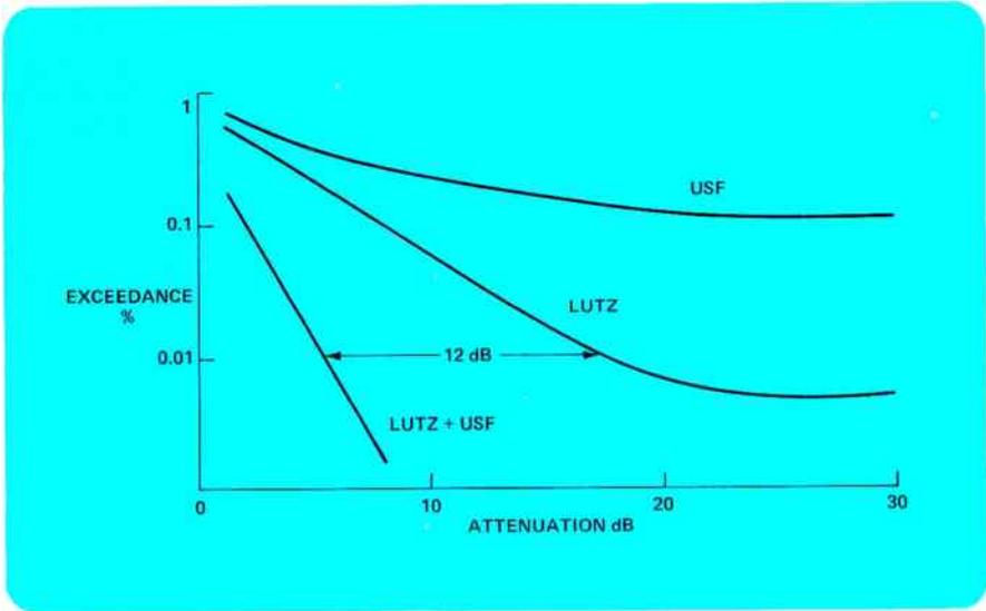
Figure 6. Diversity performance of Tampa triad June 1978 - 19 GHz.
