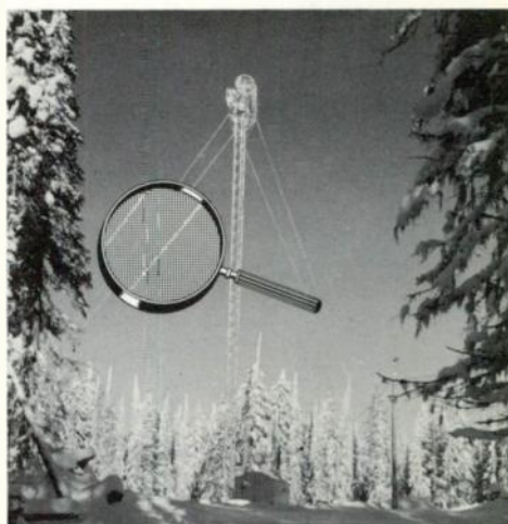
Figure 2. Printed picture illustrates how continuous shades of gray may be created using only black and white. Process is analogous to reconstructing continuous waveforms from quantized pulses.
