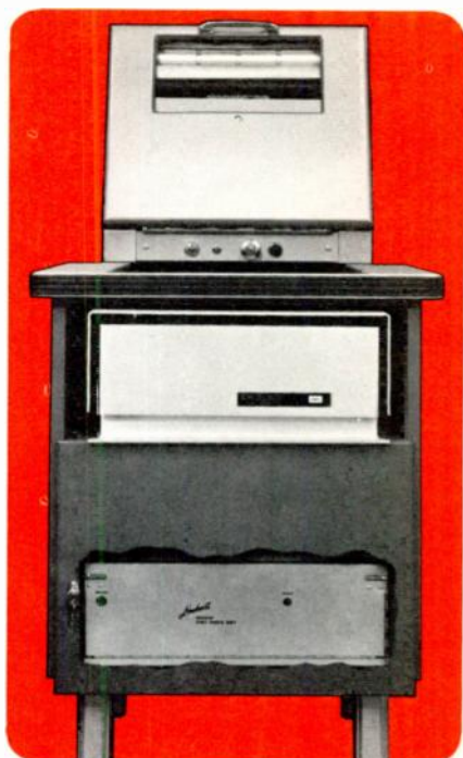
Figure 4. This black and white fax system transmitter produced by Dacom, Sunnyvale, California, makes use of Lenkurt's 26D data modem.
