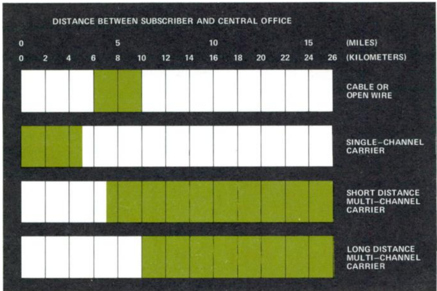
Figure 2. For relief of overloaded facilities, the green areas indicate, at the present level of technology, each system's recommended operating range.
