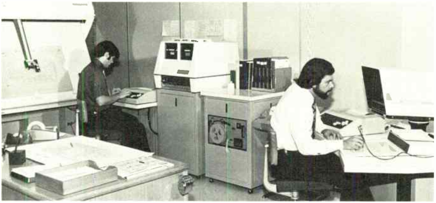
Figure 1. The automated drafting and documentation system shown has a digitizing layout table, a minicomputer, paper tape punch, and editing station. The photo plotter (not shown) is in a separate darkroom.
