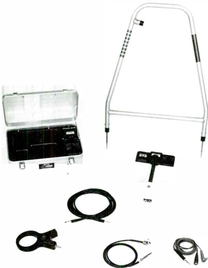
Figure 3. Sheath fault and cable locator test set.
