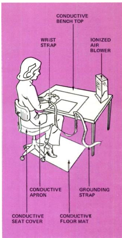
Figure 3. Typical antistatic work station showing basic requirements of grounded work surface and connected wrist strap supplemented with common auxiliary items.
