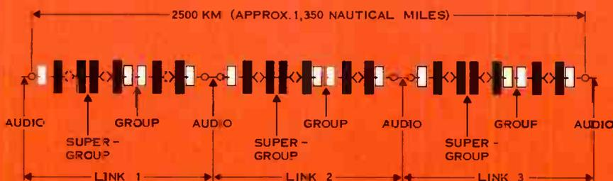
Figure 2. DCS and CCITT reference circuits.
