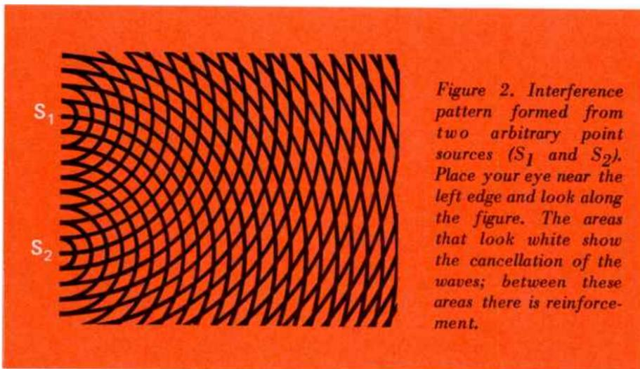
*Figure 2. Interference pattern formed from two arbitrary point sources ( $S_1$  and  $S_2$ ). Place your eye near the left edge and look along the figure. The areas that look white show the cancellation of the waves; between these areas there is reinforcement.*
