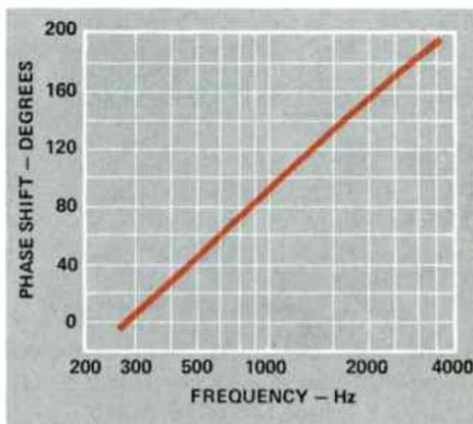
Figure 1. Cosine section phase shift-versus-frequency characteristic – Amplitude Equalizer.
