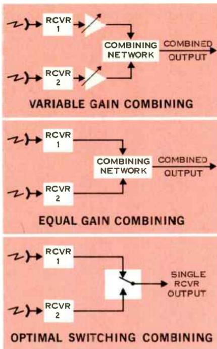
Figure 5. Some method of combining the multiple signals is required at the receive terminal of a diversity system. Three forms of combining in use are variable gain, equal gain, and optimal switching.
