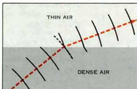
*Figure 1. The velocity of microwaves traveling through the atmosphere increases as the refractive index of the air decreases. The increased velocities at the top of the wavefront cause the microwave beam to bend.*
