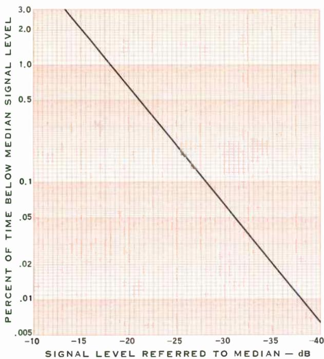
*Figure 3. Rayleigh distribution curve shows probability of fades of various depths.*
