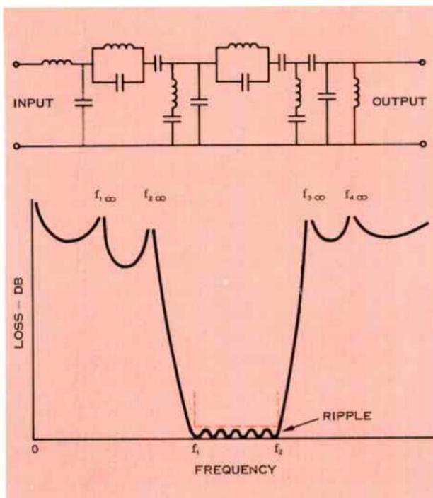
Figure 6. Filter circuit (top) will produce this type of loss-frequency curve. Engineer and computer determine optimum component values to provide proper passband frequencies, acceptable ripple, and infinite loss points.
