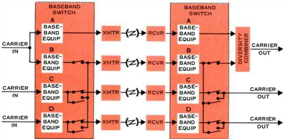
Figure 8. Block diagram of typical standby diversity protection system. Channel B operates in frequency diversity with channel A, while providing backup for channels C and D in the event of a failure.
