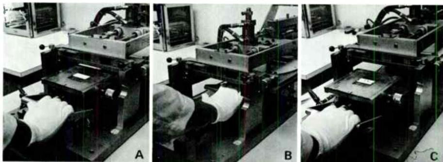
Figure 3. There are three steps in depositing the resistor pattern: (A) substrate is fitted to the vacuum chuck, (B) the substrate passes under the screen and the squeegee forces the ink through the screen and onto the substrate, and (C) the chuck is withdrawn with the pattern deposited on the substrate.
