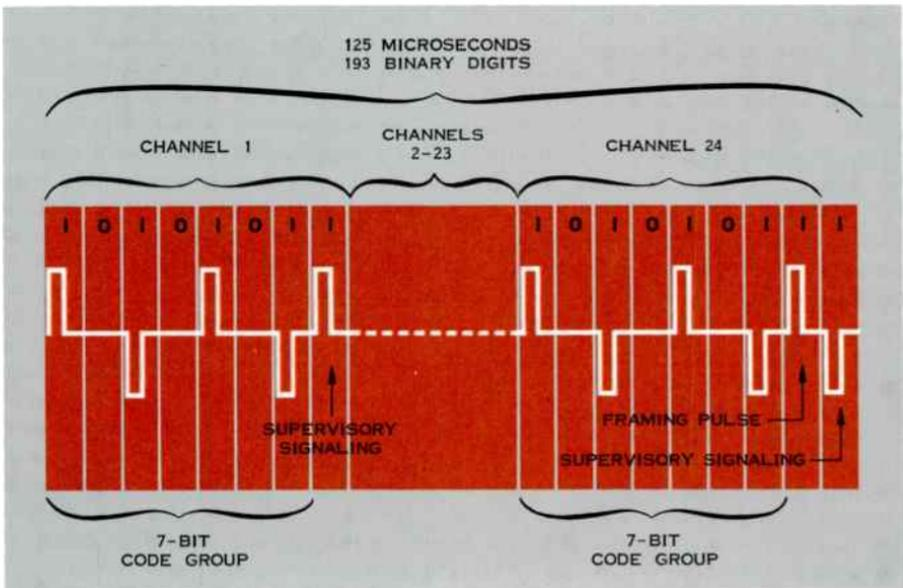
Figure 5. In the 24-channel T1 carrier system, 125 microsecond sampling interval or frame is divided into 193 time slots — 168 slots for speech, 24 slots for supervisory signaling, and 1 slot for synchronization.
