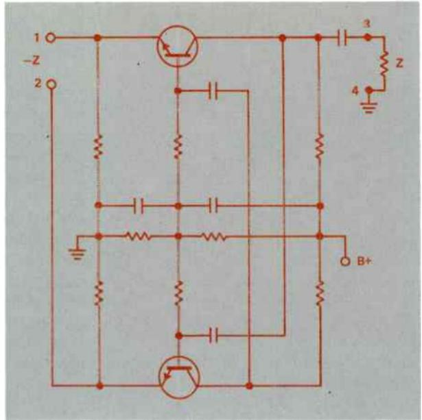
feedback in the circuit produces the negative impedance characteristics, while the negative feedback provides stability. The value of the impedance applied to terminals 3 and 4 appears at terminals 1 and 2 as the negative of that value. In practice, terminals 1 and 2 are effectively connected in series with the two sides of a telephone line and present to the line a series, or voltage-type negative impedance (Fig. 5).
