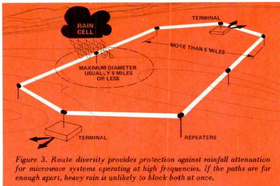
*Figure 3. Route diversity provides protection against rainfall attenuation for microwave systems operating at high frequencies. If the paths are far enough apart, heavy rain is unlikely to block both at once.*
