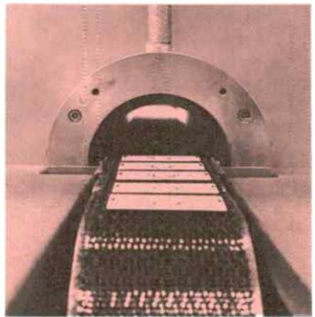
*Figure 5. The conveyor type furnace can produce firing temperatures up to 1500°C.*
