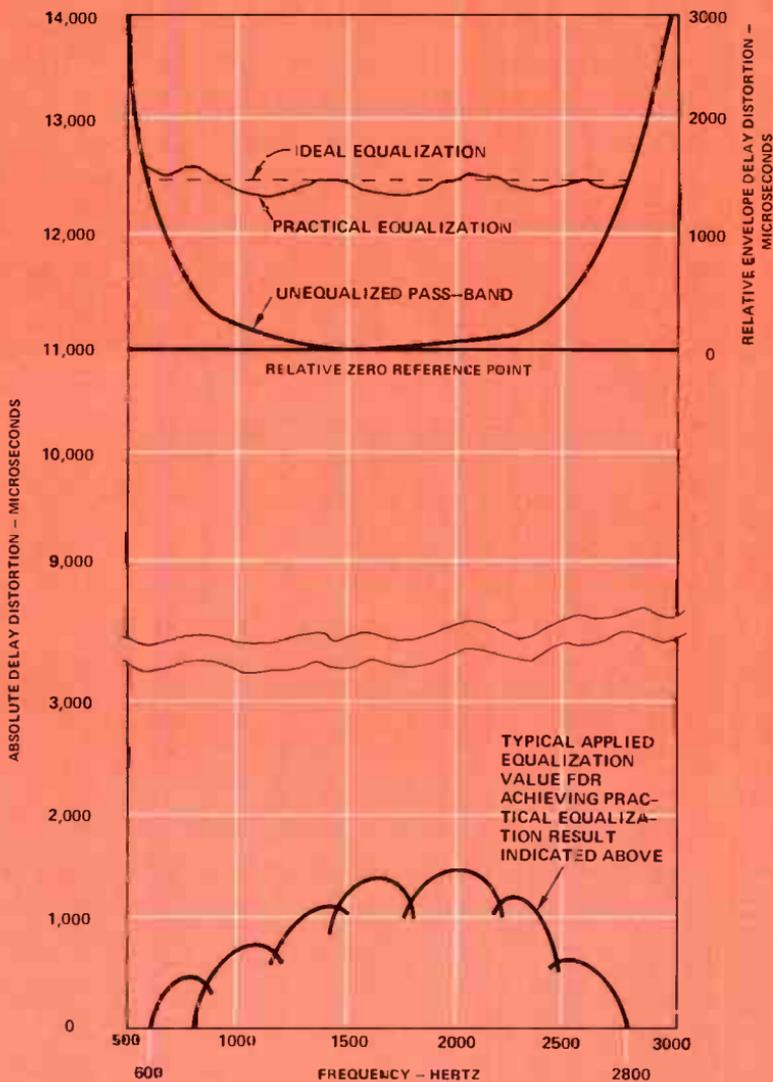
Figure 6. Relationship of Relative Envelope Delay Distortion To Absolute Delay Distortion.
