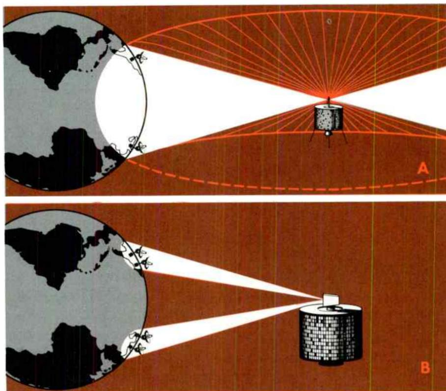
Figure 2. Early Bird employs a toroidal transmission pattern (A) which loses much rf energy to space. The proposed INTELSAT IV satellites will employ a more sophisticated and efficient transmission pattern (B).
