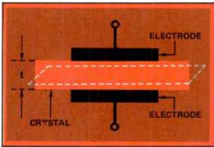
Figure 6. The dotted line shows the thickness shear mode of vibration in an AT cut crystal.
