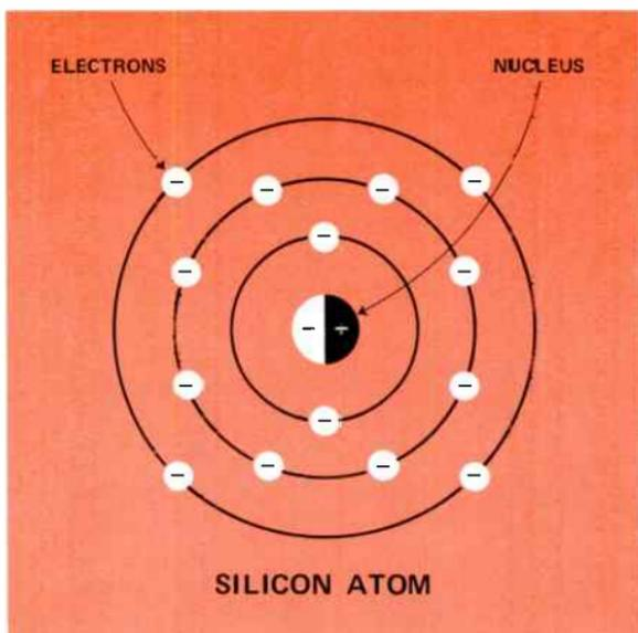
Now, if a foreign substance whose atoms have an odd number of valence electrons — say 5 — is added to the silicon, four of them will pair with the four host electrons. The fifth, or odd electron will remain free to move about in the compound and carry electric current. See Figure 2.
