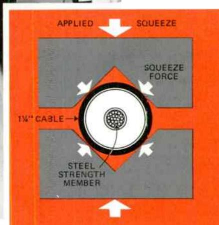
Figure 4. End view of cable engine as repeater enters engine. Insert shows how tracks grip a piece of cable. When repeater goes through, the flexible tracks separate to give the necessary clearance.
