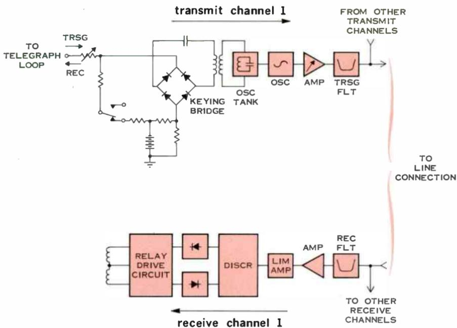
Figure 3. Simplified schematic diagram of telegraph multiplex terminal operating into a half-duplex neutral loop.
