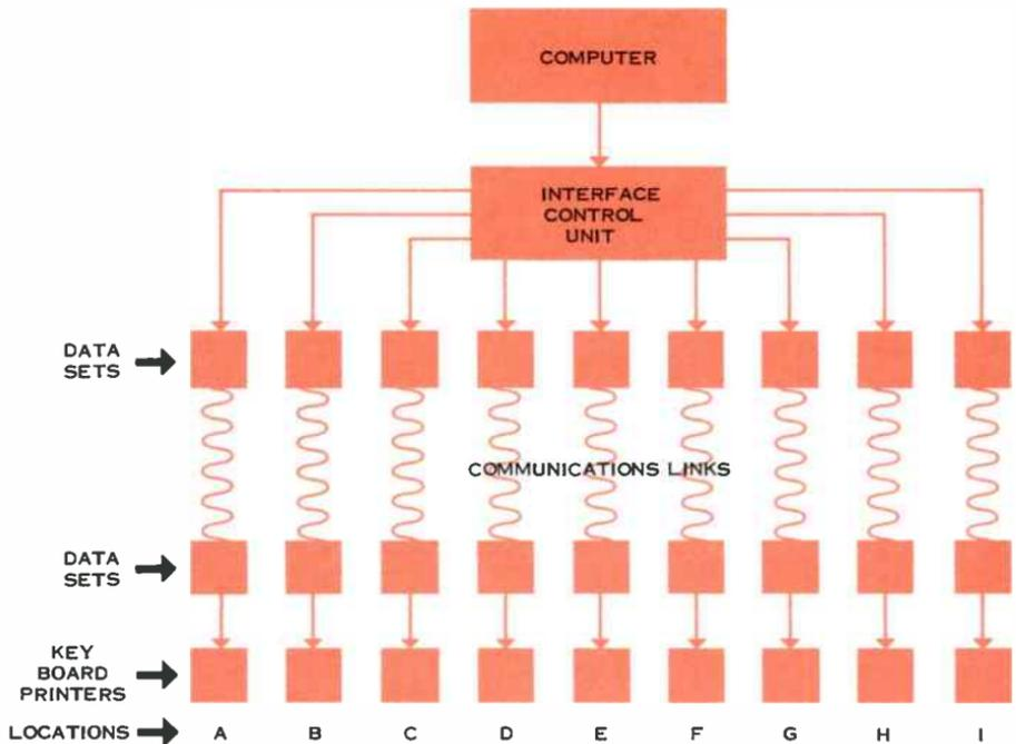
Figure 3. A typical time sharing computer employs an interface control unit to apportion its time among many users at different locations.
