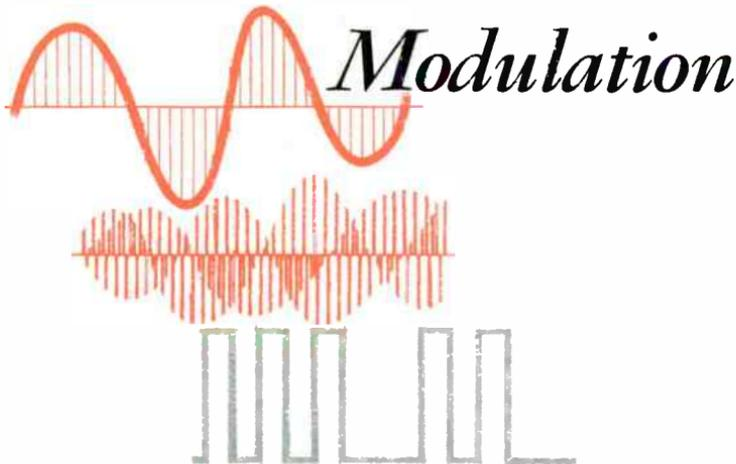
*The constant search for better communications at lower cost has led the telephone industry to a radically different method of transmitting speech information. This method, using binary digital pulses rather than conventional analog signals, provides high quality transmission and has proven to be very economical in short-haul carrier systems.*
