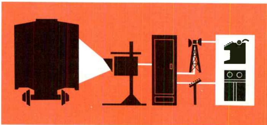
*Figure 1. The basic ACI system consists of three components — the label (on the car), the scanner and the decoder. Optional equipment can be added to meet requirements for higher levels of system sophistication.*
