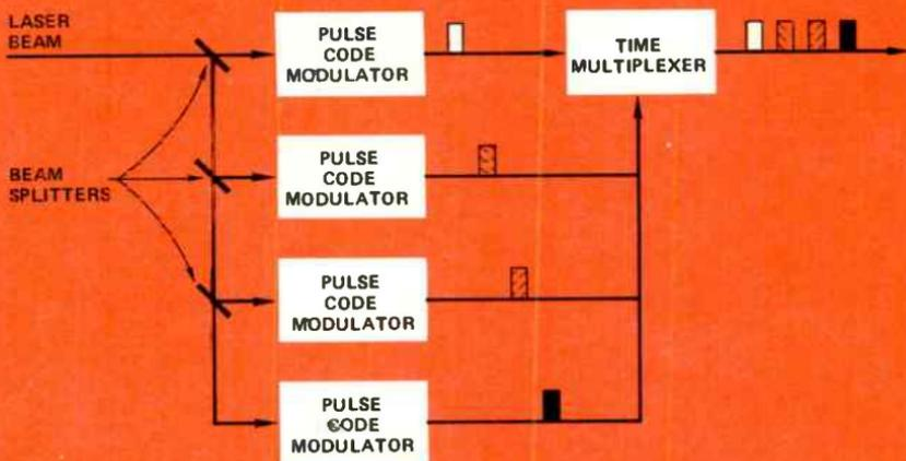
*Figure 5. PCM shows considerable promise for modulating lasers. The beam-splitting arrangement shown here forms several high-speed channels from a single laser beam.*
