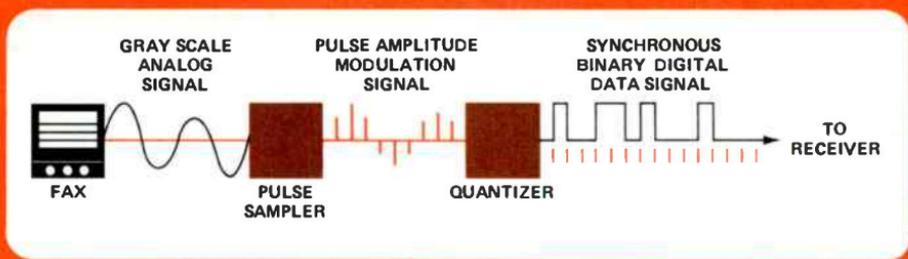
*Figure 1. By using a "sampling" device, a continuous, analog signal can be converted into a synchronized, pulse amplitude signal. This signal can further be quantized and encoded into binary digital form.*
