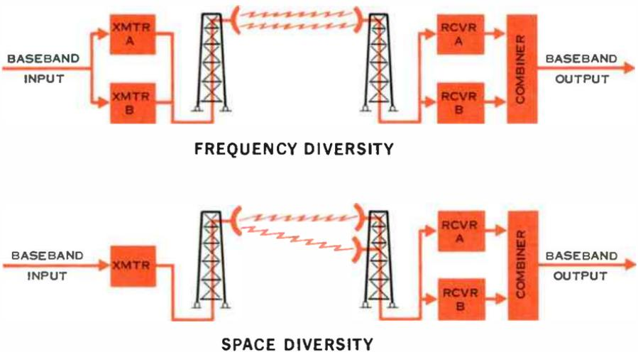
Figure 4. Two types of diversity reception commonly used in line-of-sight microwave systems are frequency diversity and space diversity.
