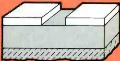
Window etched through silicon dioxide to expose epitaxial layer to diffusion.
