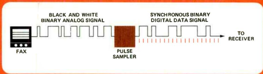
Figure 2. A "sampling" device applied to a black-and-white, binary signal, produces a synchronous, digital binary signal in one step. The binary nature of this mode effectively lowers transmission noise but introduces "jitter".
