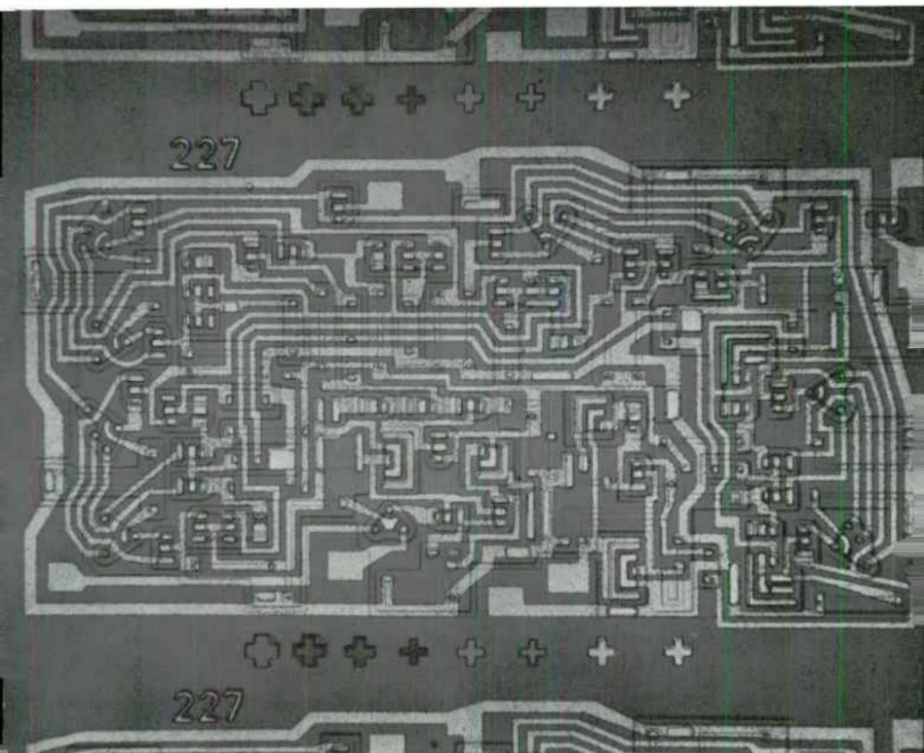
*Figure 7. Sylvania IC contains 116 transistors, resistors and diodes to produce 40 gate circuits on each chip. Used in computers or digital communications equipment.*
