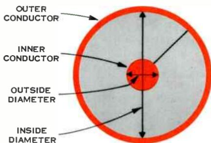
*Figure 2. Coaxial tube dimensions are specified by the outside diameter of the inner conductor, and the inside diameter of the outer conductor.*
