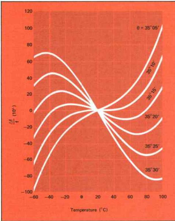
Figure 5. An AT cut crystal with an angle of  $35^{\circ} 10'$  has the best frequency stability.
