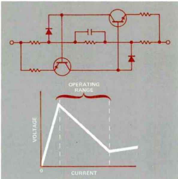
*Figure 6. Bell negative impedance booster (NIB) operates in series with the line and is powered over the cable. Slope of the operating curve is stabilized by transistor emitter feedback. Diodes add to the operating linearity.*
