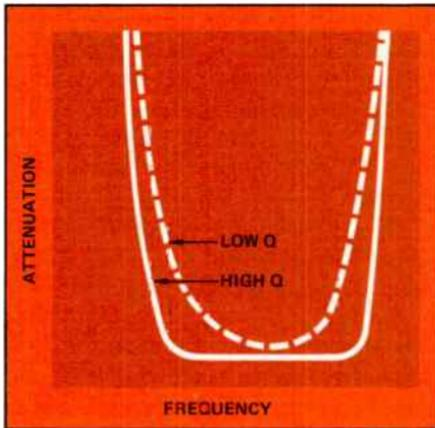
Figure 2. These curves show the passbands of the same filter made with resonators having different  $Q$  values. Note that high  $Q$  values must be used if the filter is to have a flat passband with sharp corners.
