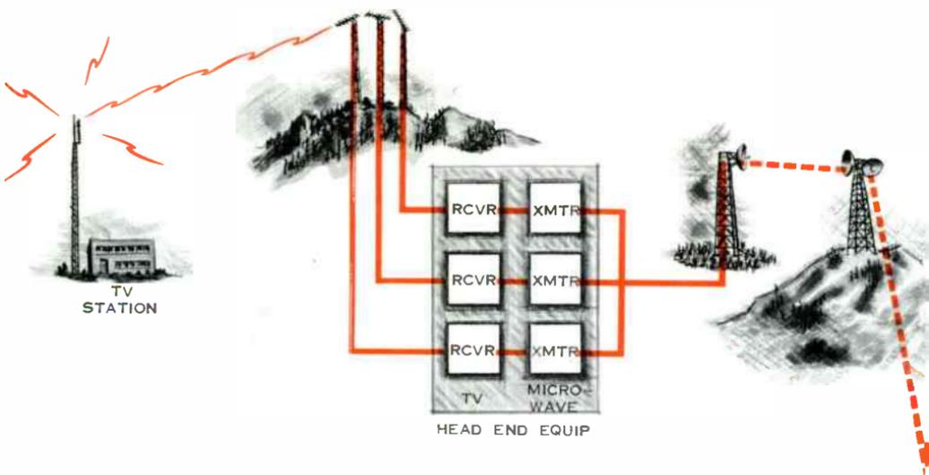
Figure 5. CATV system picks up signals outside the reach of home antennas; may use microwave radio to relay them to cable distribution point. Utility poles carry coaxial cables through residential areas.
