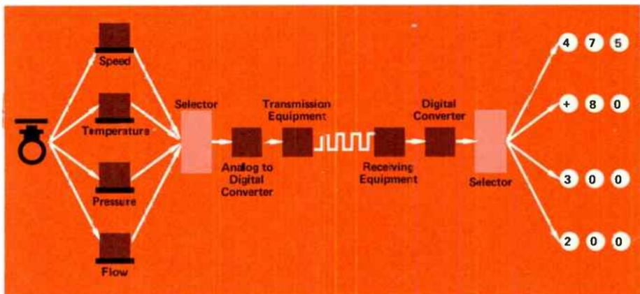
Figure 1. Simplified diagram of a typical supervisory control system.
