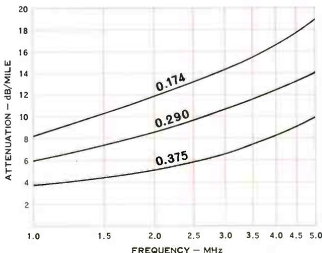
Figure 3. Response curves compare the attenuation versus frequency characteristics of the common types of communications coaxial cable.
