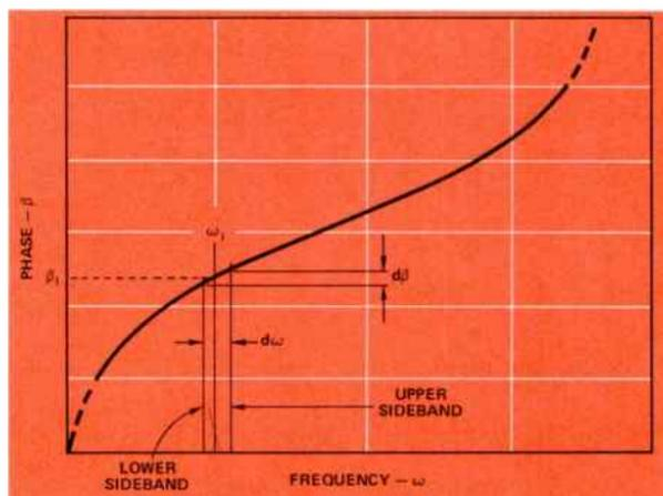
phase curve describing the circuit at the carrier frequency. (See Figure 2). This means that if the amplitude modulated test signal is tuned or swept across the band of interest, the envelope phase shift detected at the receiving end of the circuit provides an indirect measurement of the frequency/phase shift characteristics of the circuit. A curve of envelope delay-versus-frequency for a typical communications circuit is shown in Figure 3.
