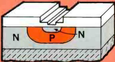
Repeated etching and diffusion create other parts of device. NPN areas now form a transistor.
