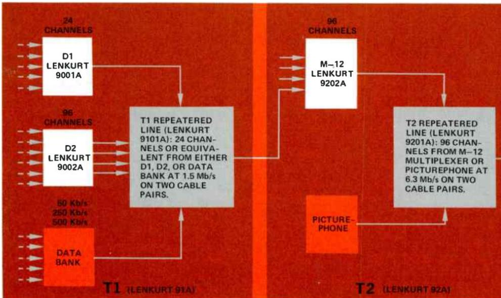
Figure 2. PCM systems, expanding from T1 to T4, will mix voice and oth
