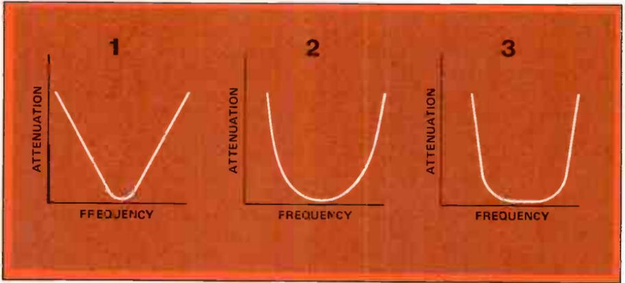
Figure 4. Each successive stage of a monolithic crystal filter improves the performance. The curves shown illustrate the successive improvement for three stages of a monolithic filter.
