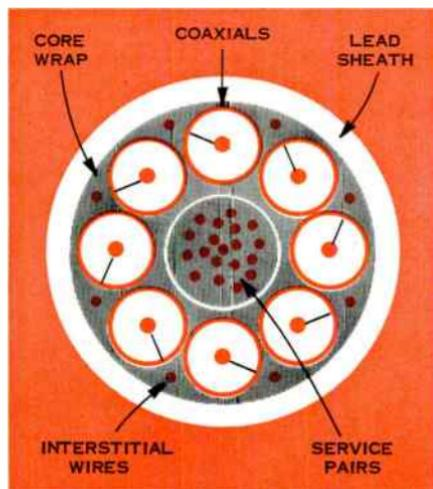
*Figure 1. Typical communications coaxial cable consists of a number of "pipes" or "tubes" together with interstitial wires and service pairs inside a single sheath. Each pipe or tube provides one-way transmission for a large number of message channels or a TV signal.*
