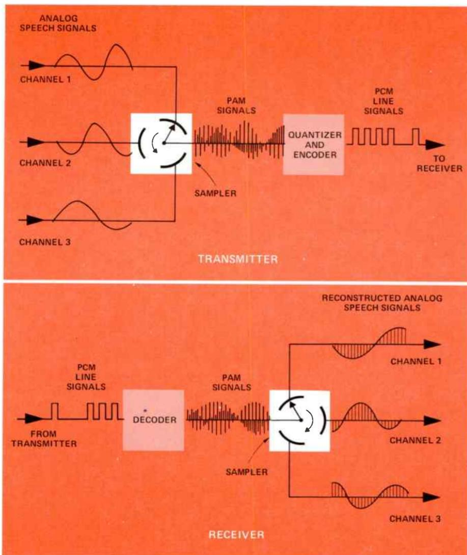
Figure 12. Simplified PCM system (only 3 of the 91A's 24 channels are shown).
