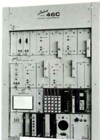
*Figure 5. Up to 600 v-f channels may be processed by office arrangement of Lenkurt 46C Coaxial Transmission System shown above.*
