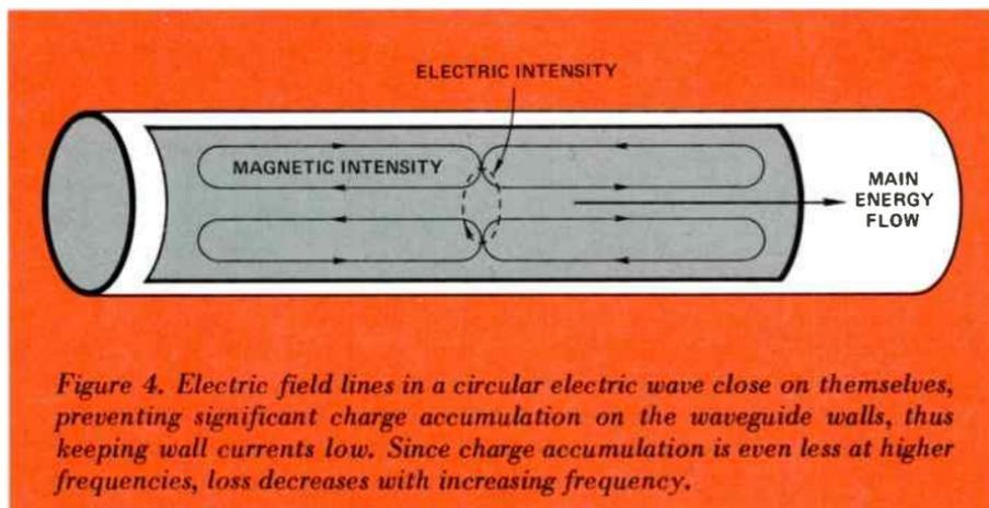
*Figure 4. Electric field lines in a circular electric wave close on themselves, preventing significant charge accumulation on the waveguide walls, thus keeping wall currents low. Since charge accumulation is even less at higher frequencies, loss decreases with increasing frequency.*
