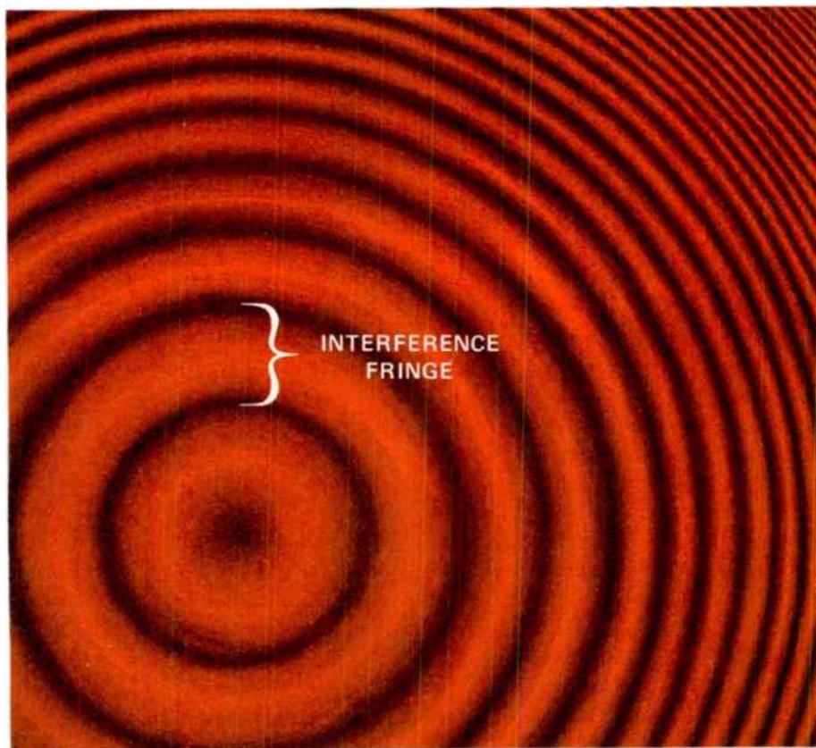
*Figure 3. A concentric ring, diffraction grating, for one point on the object, covers the entire holographic plate. The center of the grating need not be on the holographic plate. Such a grating, with variable spacing, focuses the light falling on it at a particular point.*
