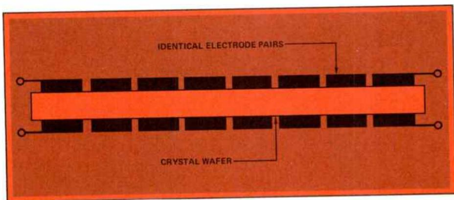
Figure 3. A monolithic crystal filter is a single crystal wafer with acoustically coupled resonators formed by plating identical electrode pairs on the crystal surface. Crystal filters are bi-directional; therefore, either end may be used as input or output.
