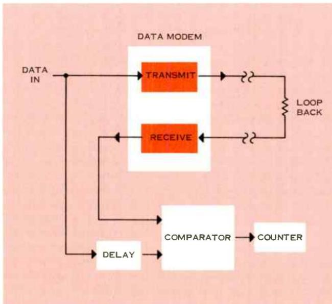
Figure 2. Typical method for measuring error performance of a data communications set. Data signals are looped back from transmitter to receiver. Delay corresponding to the amount in the path is added to the original data signals which are then compared bit-by-bit with the received data signals. An error counter keeps track of the number of errors.
