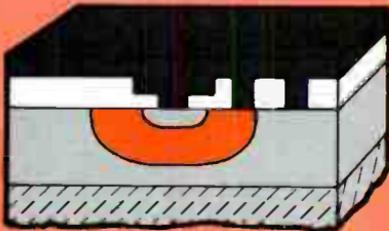
New windows are cut for placement of leads. Surface is covered with metal, typically aluminum.
