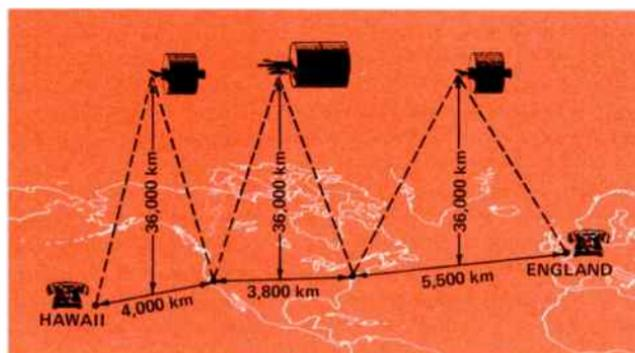
*Figure 5. Limiting intercontinental communications to one up-and-down link, there are several possible routes for a call from England to Hawaii.*
