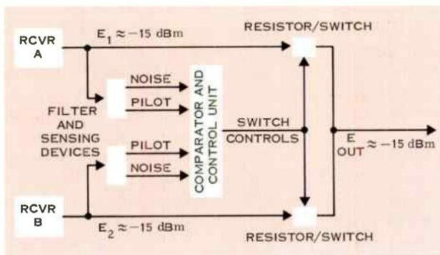
Figure 7. Simplified diagram of typical combination equal-gain optimal-switching combiner circuit.
