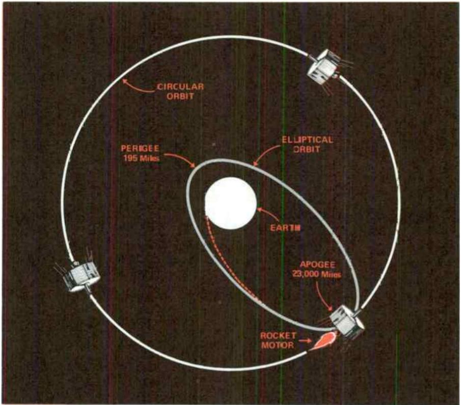
*Figure 1. Accomplishing a synchronous, geo-stationary orbit requires the satellite be launched in an elliptical orbit, whose apogee approximates 22,300 statute miles. When the satellite approaches this point an apogee rocket motor, on command from the ground, is fired replacing the satellite in "fixed" orbit. Additional thrusters are employed from time to time to maintain proper attitude and earth alignment.*
