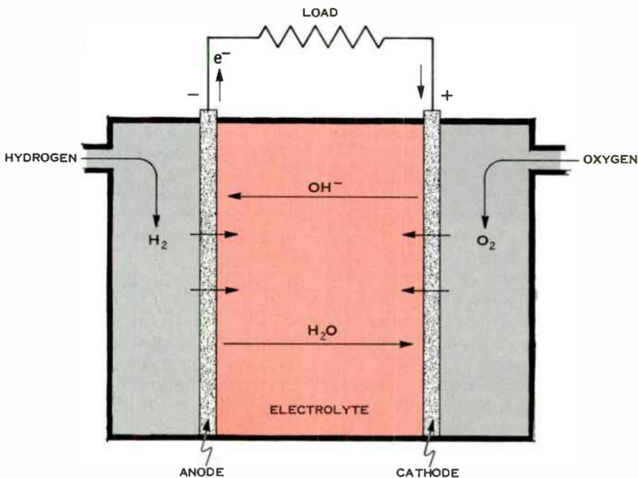
*Figure 2. At the anode of the hydrogen-oxygen fuel cell, hydrogen joins with hydroxyl ions to produce water, freeing electrons to do work. At the cathode, oxygen reacts with water in the electrolyte and electrons from the external circuit to form hydroxyl ions.*
