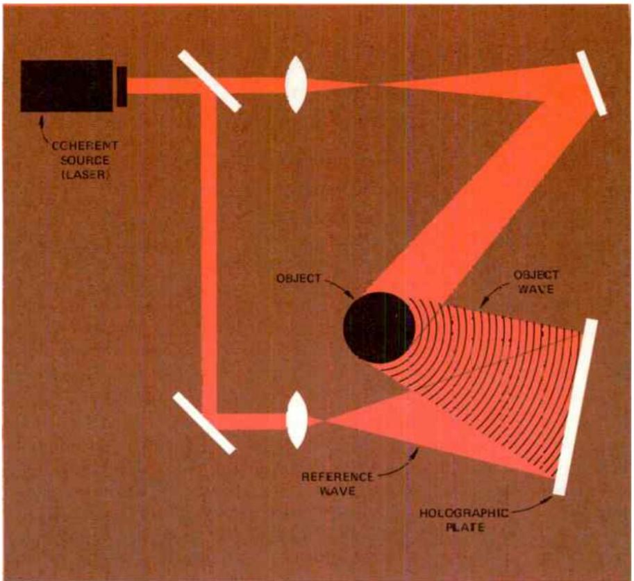
*Figure 1. Holographic recording process using laser illumination. The laser beam is split, with the object waves illuminating the object and the reference wave providing a coherent background. The two waves interfere at the holographic plate forming the hologram.*
