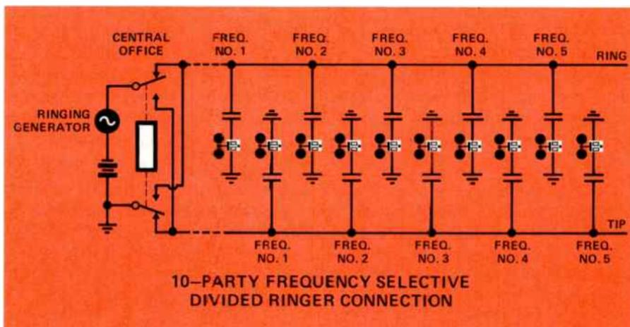
Figure 5. For ten-party frequency-selective service two sets of frequencies, either decimonic, harmonic or synchronomic, are used with divided ringer connections.
