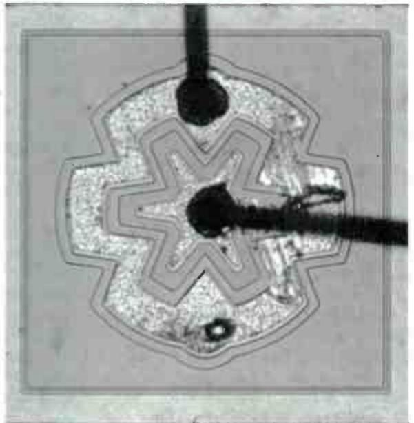
Figure 8. Using star geometry, semiconductor manufacturers are able to increase the peripheral length of the transistor. This enables it to handle greater power and current loads and still maintain low input and output capacitance.
