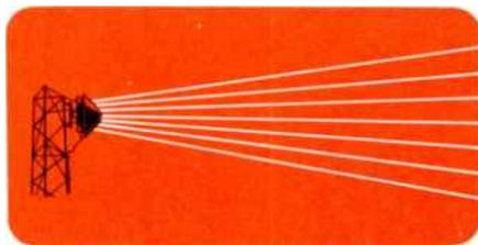
*Figure 5. Radio signals spread as they travel through the atmosphere. In effect the signal becomes many beams each subject to the atmosphere's influence.*
