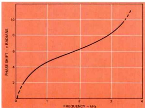
*Figure 1. Frequency/Phase Shift Characteristic's of Typical Communications Channel.*
