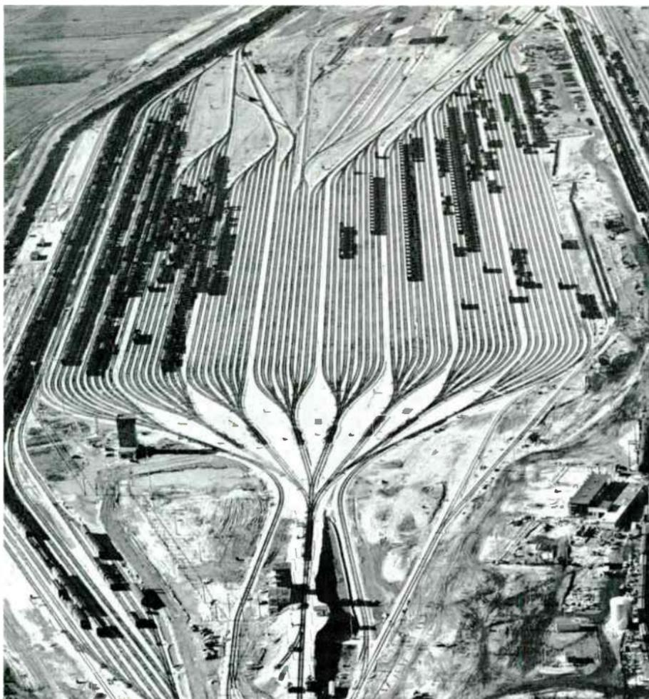
*Figure 7. The complexity of marshalling yards such as this one illustrates the need for automatic car identification.*
