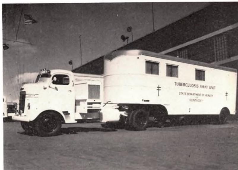
Figure 5—Self-contained, trailer-mounted chest survey unit.
