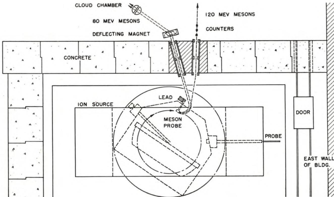
**Figure 3 — Plan view of the cyclotron, showing proton and meson trajectories.**
