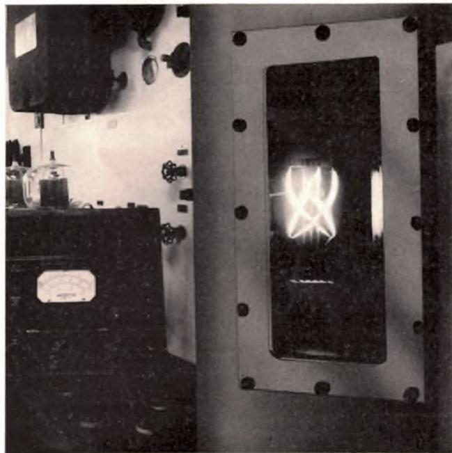
Figure 2 — Equipment Used In Carburization of ML-199 Filaments.
