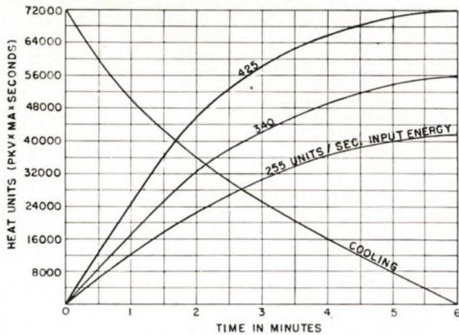
Figure 3 — Anode thermal characteristics chart for Dynamax "26."
