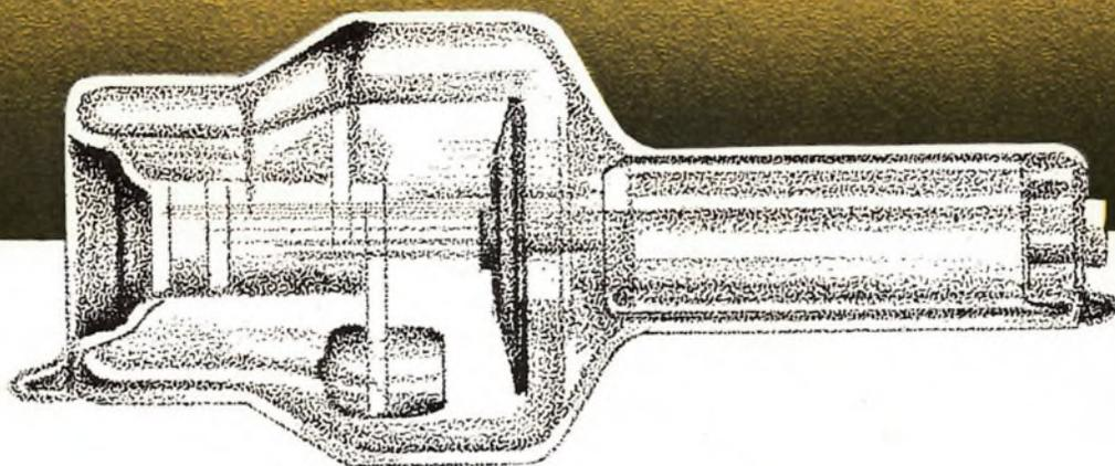
tures, this vaporizing process can last for 1000 to 2000 hours before the tube becomes unusable. This boiling off of tungsten in the form of tungsten vapor follows a natural law that is directly related to time and temperature only and is not influenced by other considerations. In other words, the filament vaporizes away without regard to any other function of the tube, assuming, of course, that the tube has been properly
