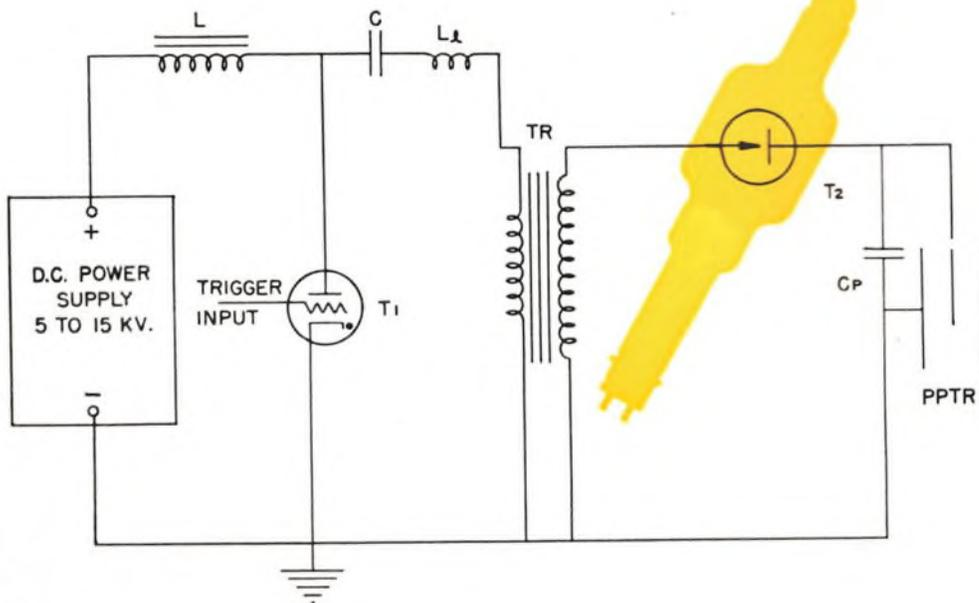
Figure 6 — Schematic Drawing of Pulsar For Supplying High-Voltage Power in Electrical Precipitation.
