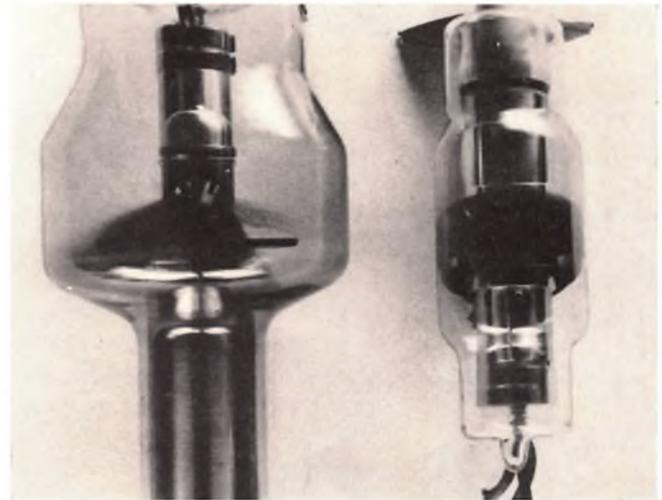
Figure 4 — Tungsten vapor deposit on glass envelope of x-ray tubes indicating excessive filament temperature.
