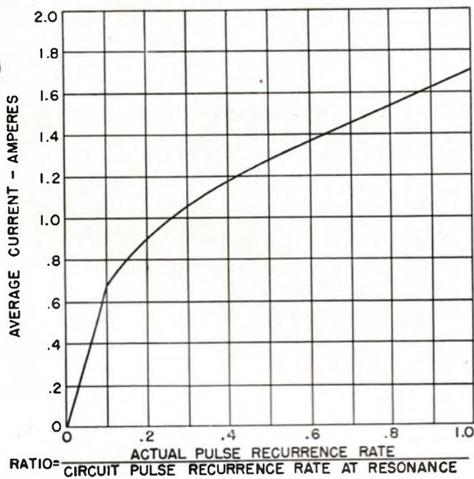
Figure 5 — ML-199 Average Current For Resonant Charging in Pulsar Circuits.
