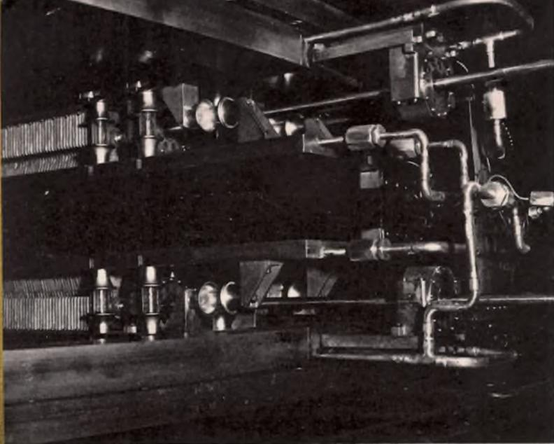
**Figure 2 — Interior of the vacuum chamber and two rotating condensers.**
