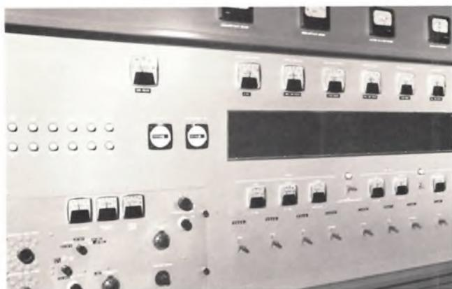
Control panel of the General Electric vapor-cooled 250 kW transmitter. Extremely compact for its power capability, this new transmitter employs five ML-7482 triodes: two as modulators, one in the second intermediate power amplifier position; and two as rf power amplifiers. (An extensive description of this transmitter may be found in CATHODE PRESS, Volume 19, Number 1, 1962.)
