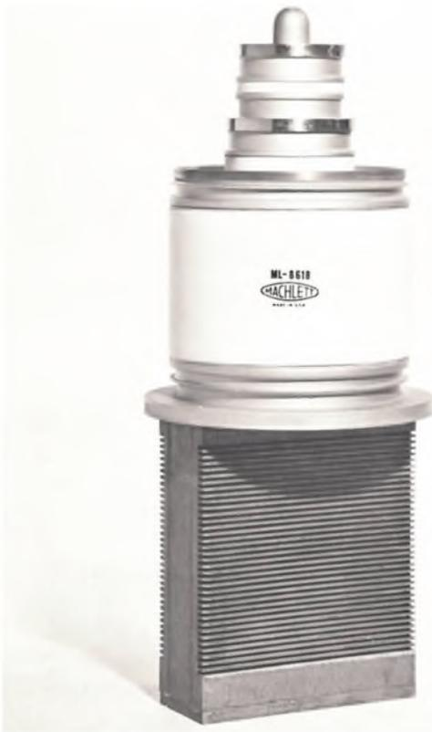
Figure 5 — Complete ML-8618 Showing Large Anode to Grid Seal Area.
