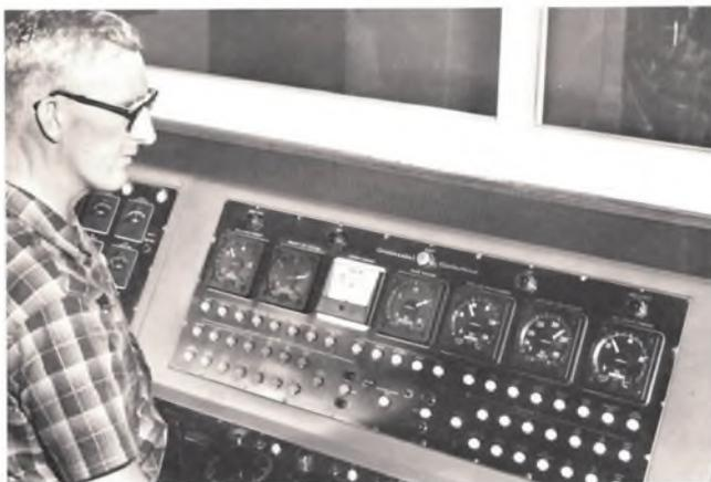
At the console of a 500 kW Continental transmitter, adjustment is made for the desired operating power — in this case, as shown below: 15 kV, 52 amperes. Continental Electronics Doherty's similar to this are in service for the VOA both here and in Europe. At Munich, for example, a 1 megawatt (carrier power) transmitter using ML-5682's has been in service for nearly 15 years. (An extensive description of this transmitter may be found in CATHODE PRESS, Volume 10, Number 1, 1953.)
