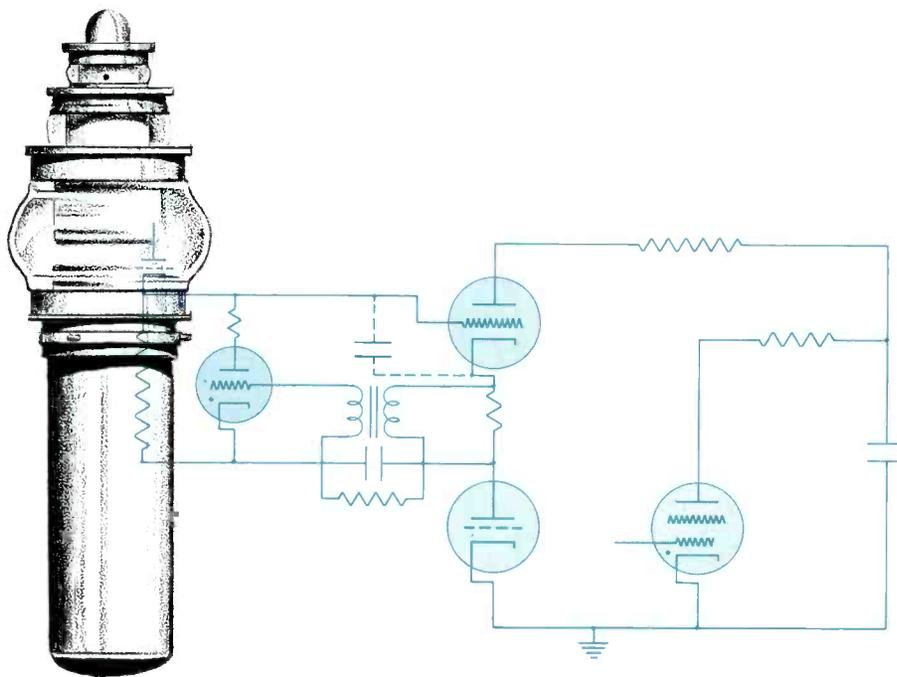
power tube to the crowbar circuit. The diverter circuit must also be capable of dissipating the power fed through until the primary circuit is opened. It should be borne in mind that crowbars are essential for good high voltage tube stability even when flash arcs are too weak to cause catastrophic damage.
