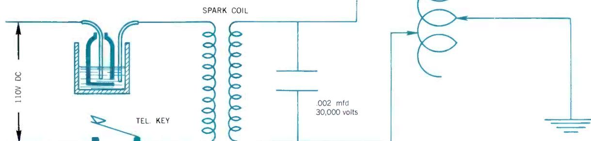
Figure 9 — Schematic drawing of the 3BV transmitter.
