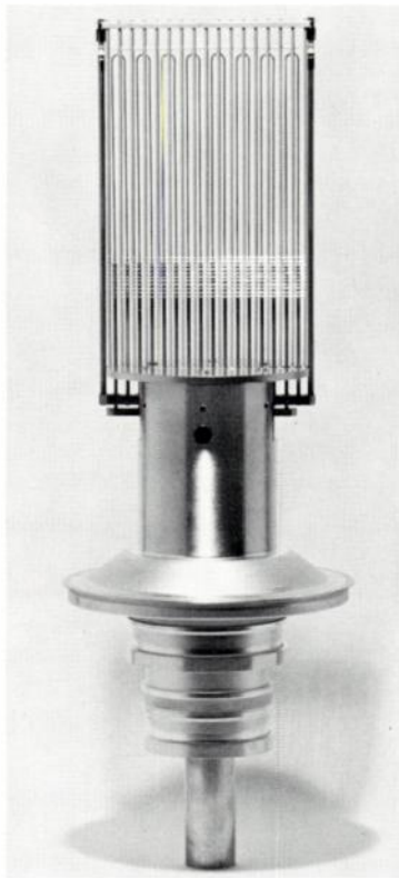
Figure 3 — Cathode-Grid-Terminal Assembly of ML-8618.
